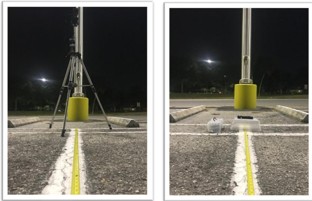
Figure 3. Measurement of Horizontal Illuminance at 5 ft 3 in. (left) and 6 in. (right)
