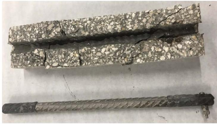
Figure 3.22: Steel reinforcement and concrete section after extraction.
