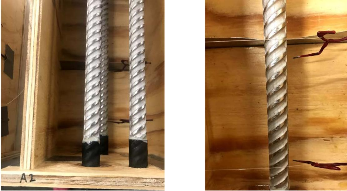
Figure 3.26: Experimental setup of reference electrodes.
