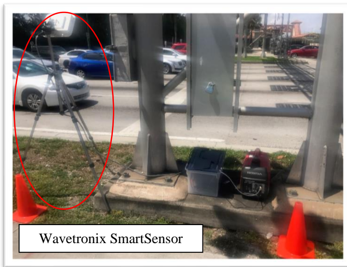
Figure 2-3 Installation of Wavetronix SmartSensor and GoPro on pneumatic mast
