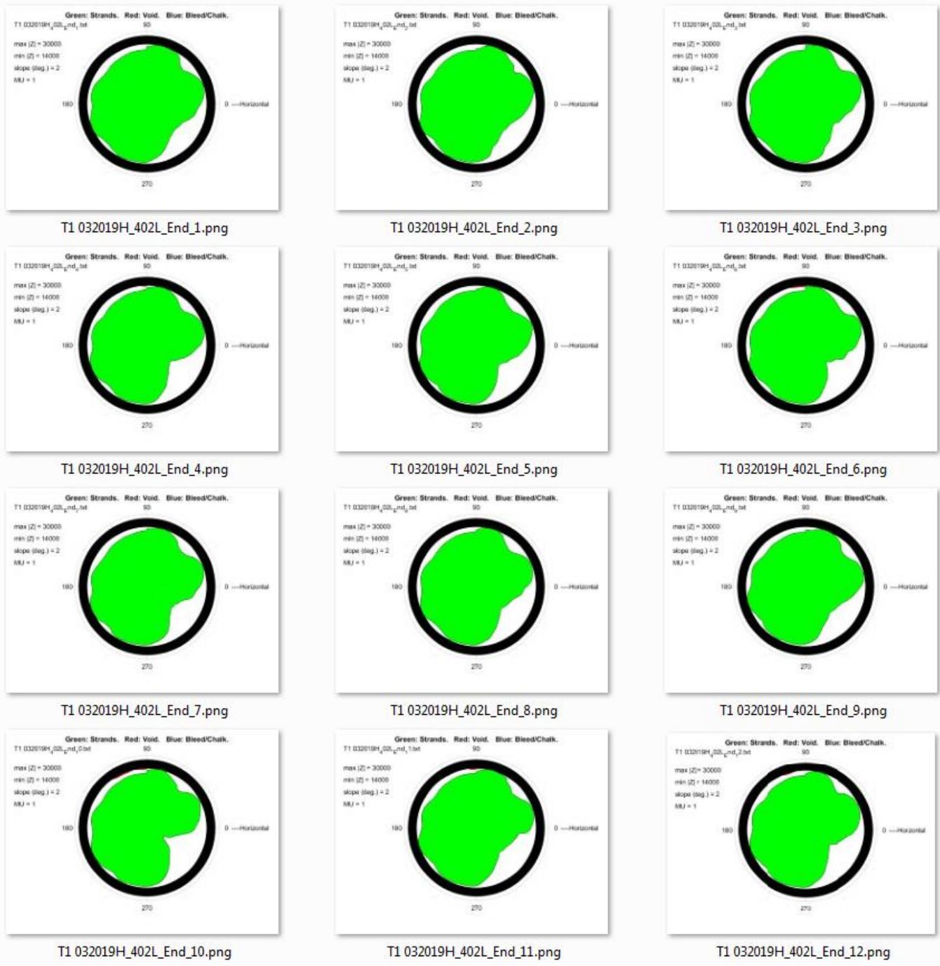
Figure 10 Images generated at Test 1 place on tendon 402L. Each row is for a group numbered as identified in the text, illustrating robustness of results to wiring and grounding variations, as well as illustrating repeatability within each condition. The strand bundle is colored green, while sound grout is white. No grout deficiencies were strongly apparent at this test place.
