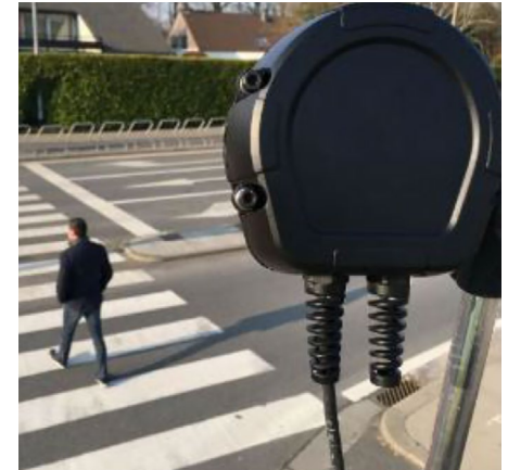
From its high perch, an automated pedestrian detector monitors corners and crosswalks for the presence of pedestrians and the need for crossing signals.
