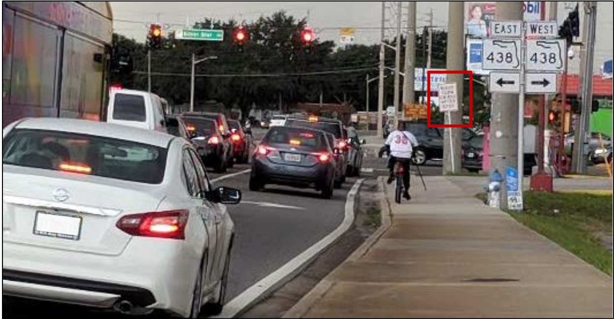
Figure 18. D5 site after implementation of “Right Turn on Red” After Stop sign
