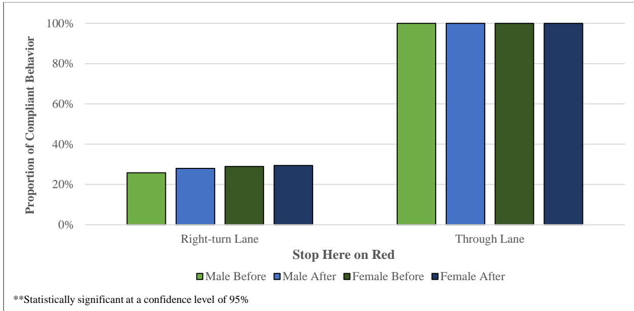
Figure 70. Comparison of compliance for “Stop Here on Red” sign by gender, District 1
