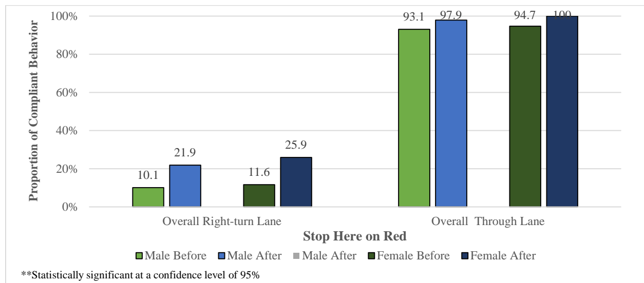
Figure 49. Comparison of compliance for “Stop Here on Red” sign by gender, Districts 1 and 7
