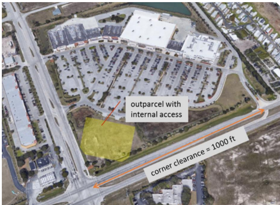
Figure 4: Corner clearance of shopping center access.
