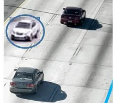
A video-based detection system must correctly detect the presence of a vehicle and its direction of travel..
