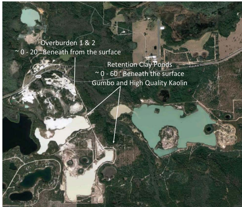
Figure 2-8: High Purity Kaolin Mine, aerial view [7]
