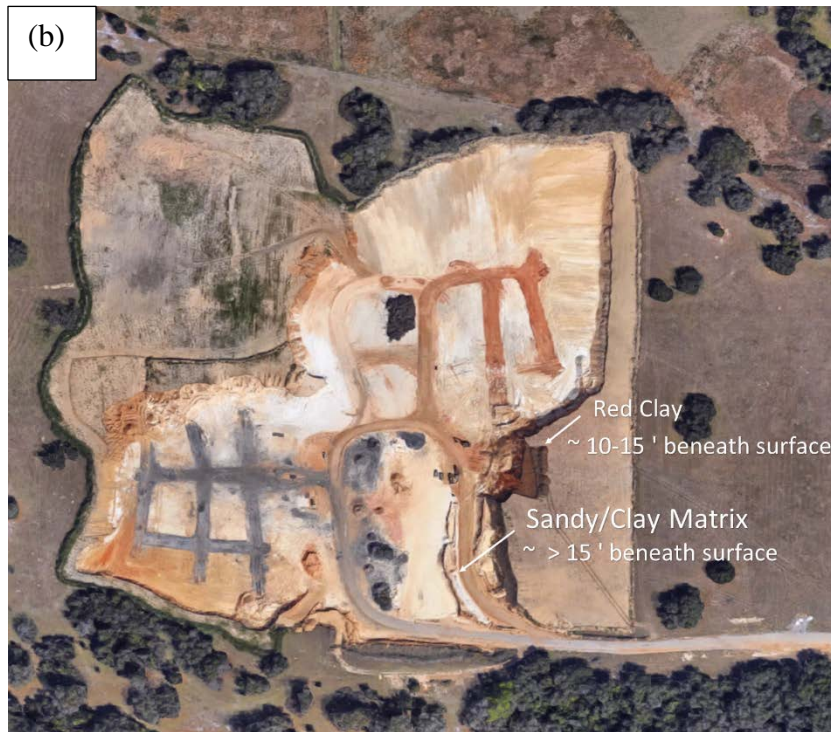
Figure 2-1: Clay Pit 168A: (a) clay stratification in the mine wall, (b) aerial view [7]
