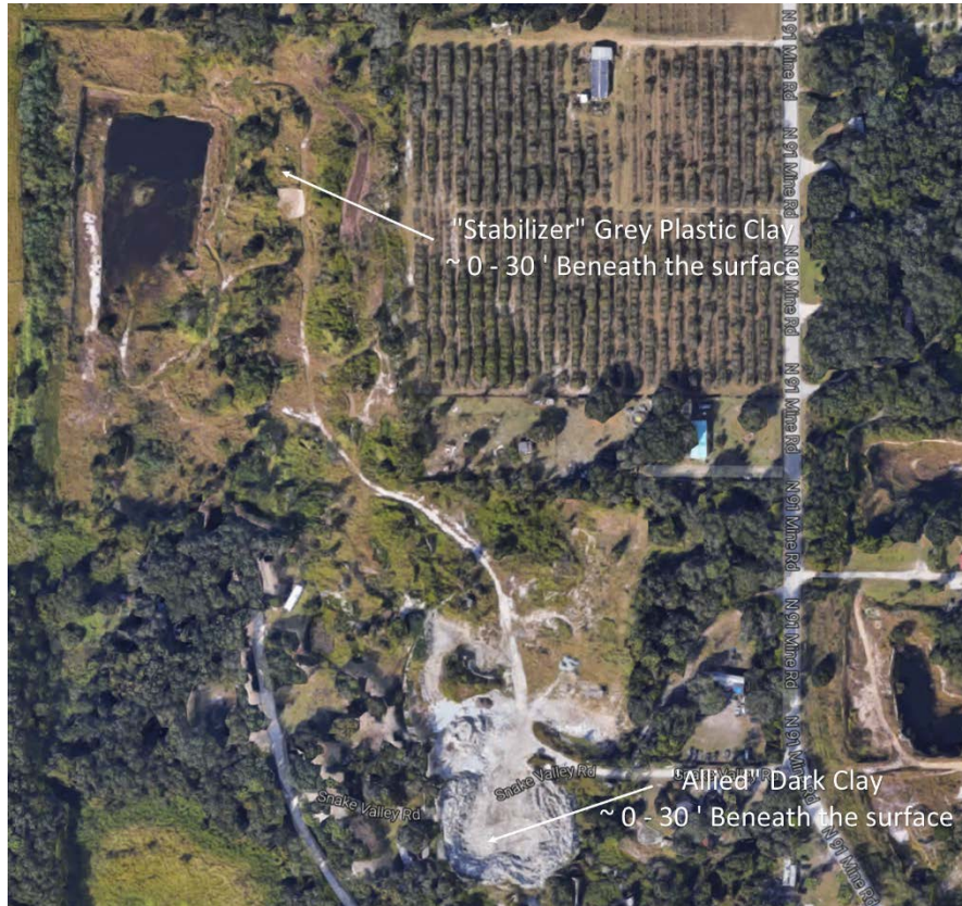
Figure 2-3: Clay Mine [7] with 2 types of clay
