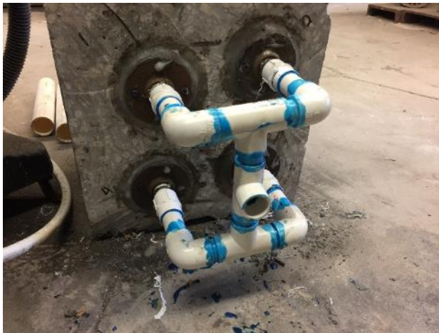
Figure 4-12: Concrete specimen 9 prepared for WD-40 injection for 24-hrs. Concrete specimen 9 with PVC manifold (lower left); specimen 9 WD-40 injection (lower right).
