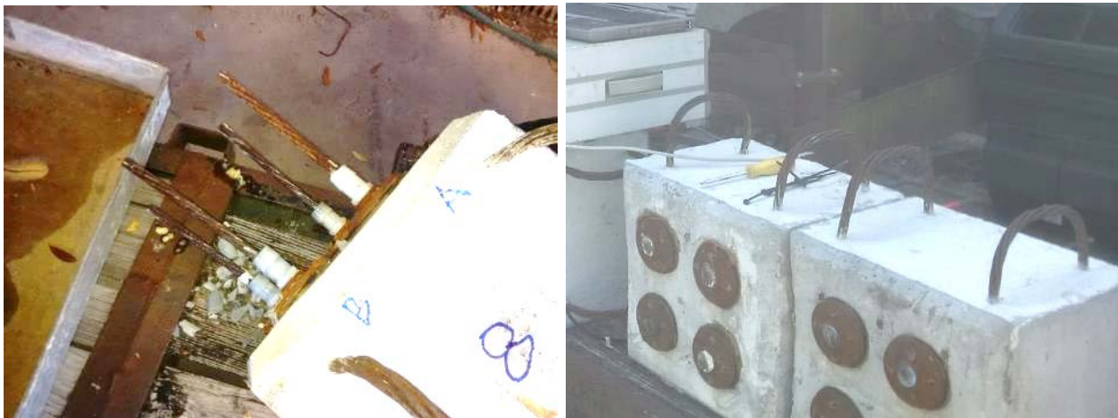
Figure 4-60: Strands extending from specimens (left); flush cut on backside (right).
