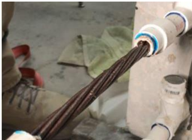
Figure 4-13: Strand coated in WD-40 (left) and extracted strand after WD-40 injection (right).
