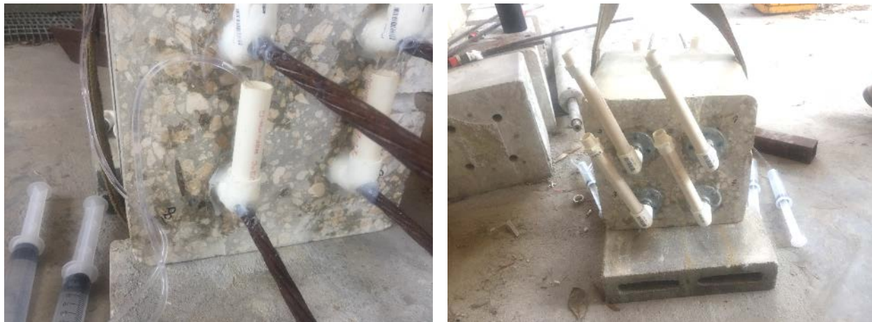
Figure 4-8: Water-filled syringe with flexible hose in the tendon (left); Back of the specimen with the standpipes and adapters (right).
