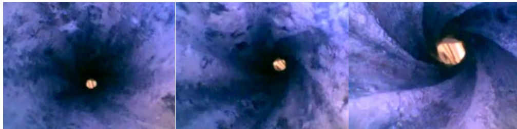
Figure 4-50: Sample 2-2 fully bonded strand, highest pullout load, 20-cc void volume.
