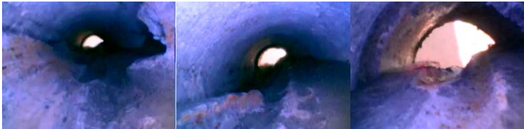
Figure 4-49: Sample 1-2 (none) 40-cc grout on only one side 2,061-lb pullout capacity.
