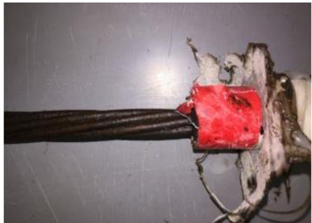
Figure 4-13: Strand coated in WD-40 (left) and extracted strand after WD-40 injection (right).
