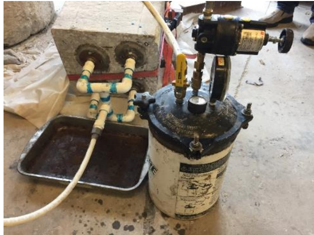
Figure 4-12: Concrete specimen 9 prepared for WD-40 injection for 24-hrs. Concrete specimen 9 with PVC manifold (lower left); specimen 9 WD-40 injection (lower right).
