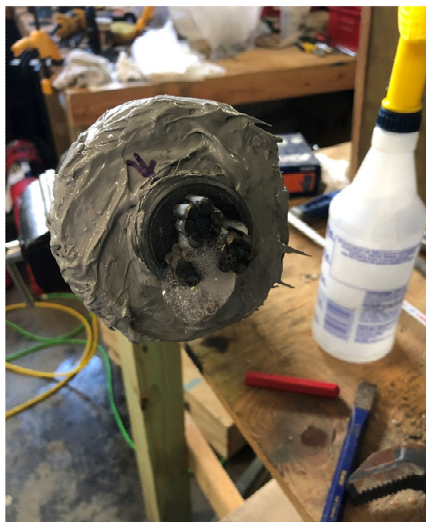
Air testing 3ft Specimen – photo shows bubbles formed by air exiting the interstitial spaces in the tendons.
