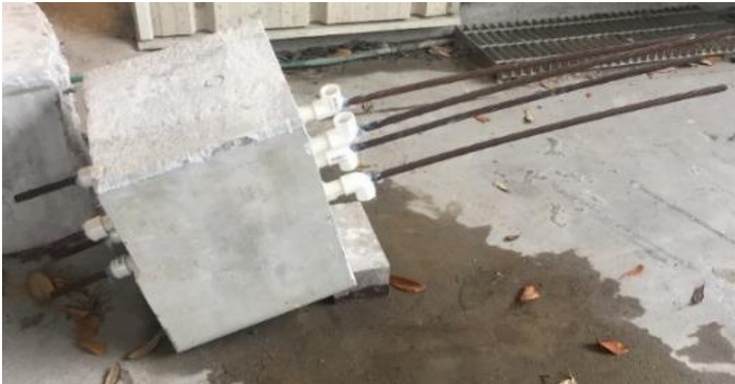
Figure 4-2: Concrete specimen 1 completely set up before grout installation
