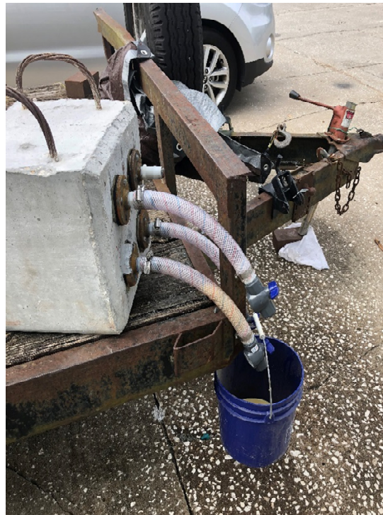
Down-stream end of tendons – photo shows two right tendons' valves closed after appearance of impregnation material. Bottom joint also shows a location of a sealed leak.
