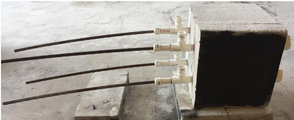
Figure 4-11: Concrete specimen 9 before grout installation.
