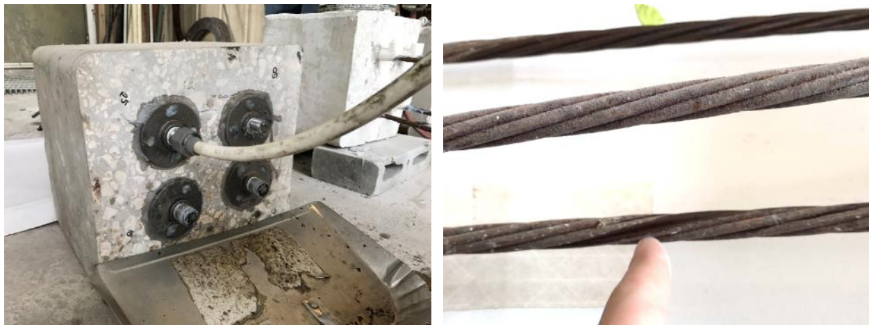
Figure 4-10: Specimen pressurized with WD-40 (left); WD-40 traveling along strand (right).
