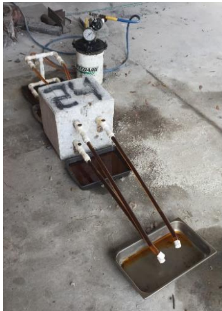
Figure 4-18: Concrete specimen 24 after 24 hrs of PB Blaster injection.
