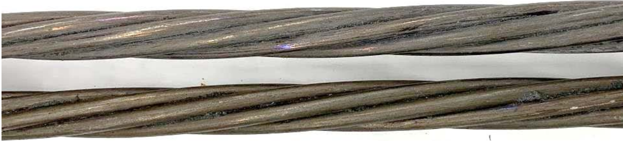
Figure 5-9: The reinforcement extracted from the 1-ft normal tendons. The reinforcement on the top is from the control group and the reinforcement on the bottom is from the impregnated group.
