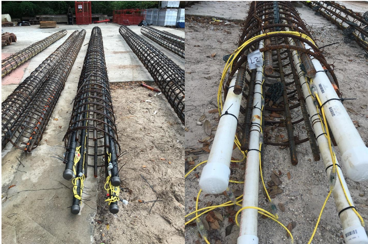
Figure 2.5 Bottom end view of reinforcement cages for 24-in piles C2 (left) and L2 (right) instrumented with thermal wires and access tubes for thermal probe testing.
