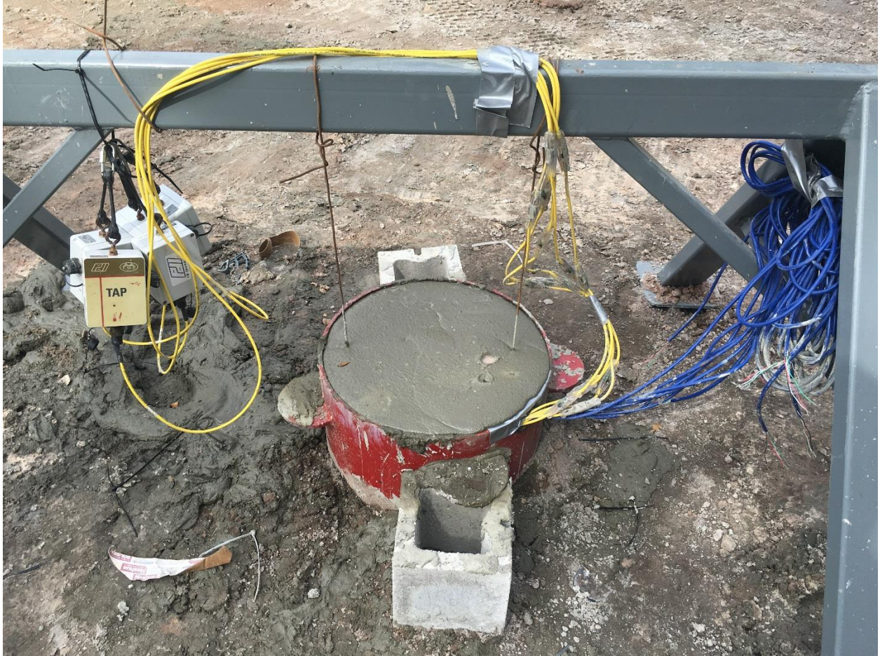
Figure 2.17 Pile C1 with thermal wires and attached TAP units.
