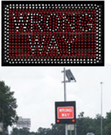
Figure 12: Detection-triggered LED Lights around “WRONG WAY” Signs
