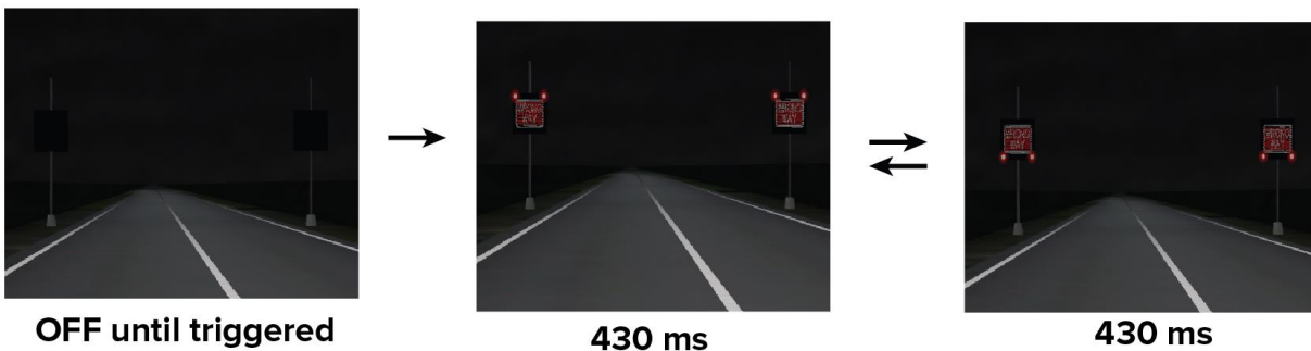
Figure E.3.11. Depiction of Flash Pattern for Countermeasure “WRONG WAY” Blank-out
