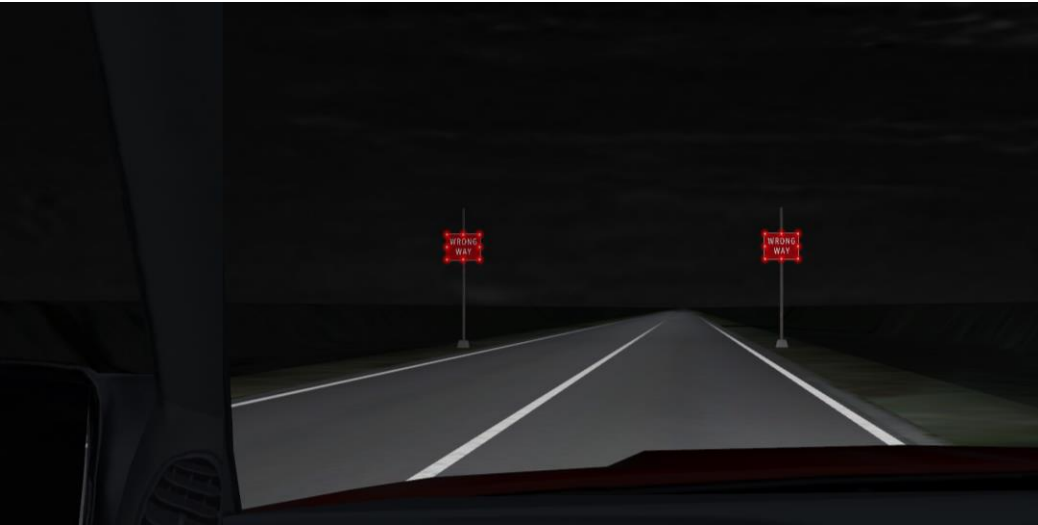
Figure 67: "WRONG WAY" LEDs
