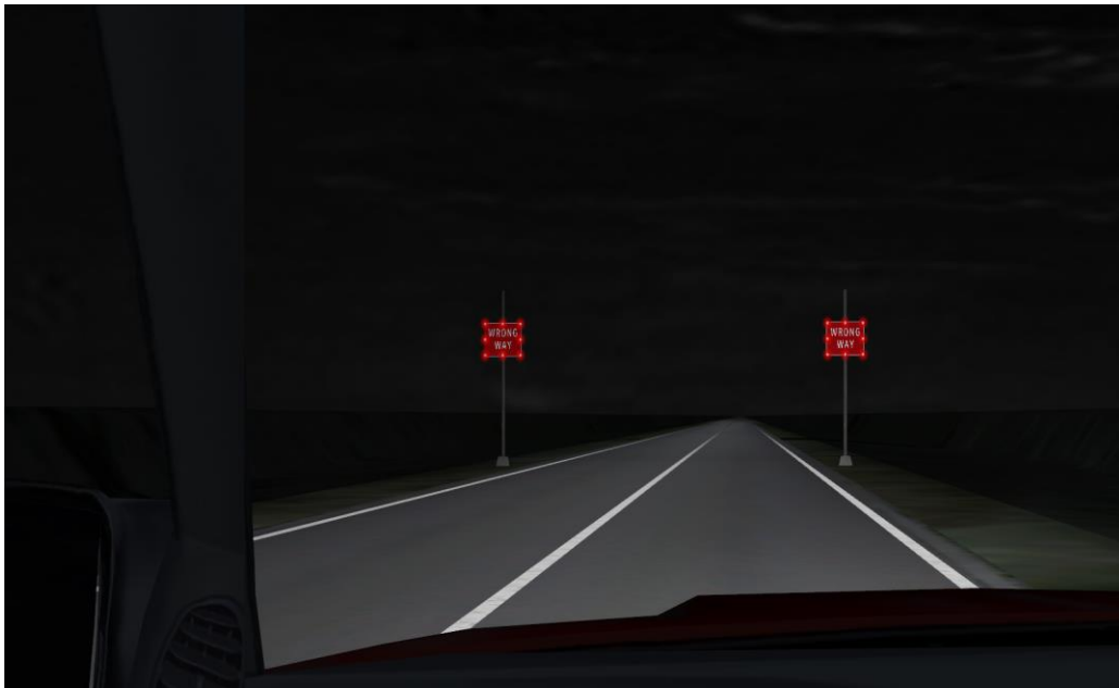
Figure E.3.5. Depiction of Countermeasure “WRONG WAY” LED
