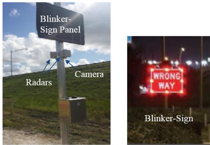
(b) LED-illuminated “WRONG WAY” sign details
