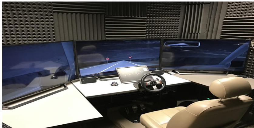
Figure 63: NADS MiniSim Driving Simulator Setup at FSU Psychology Department – Countermeasure “WRONG WAY” Blank-out Depicted on Screen
