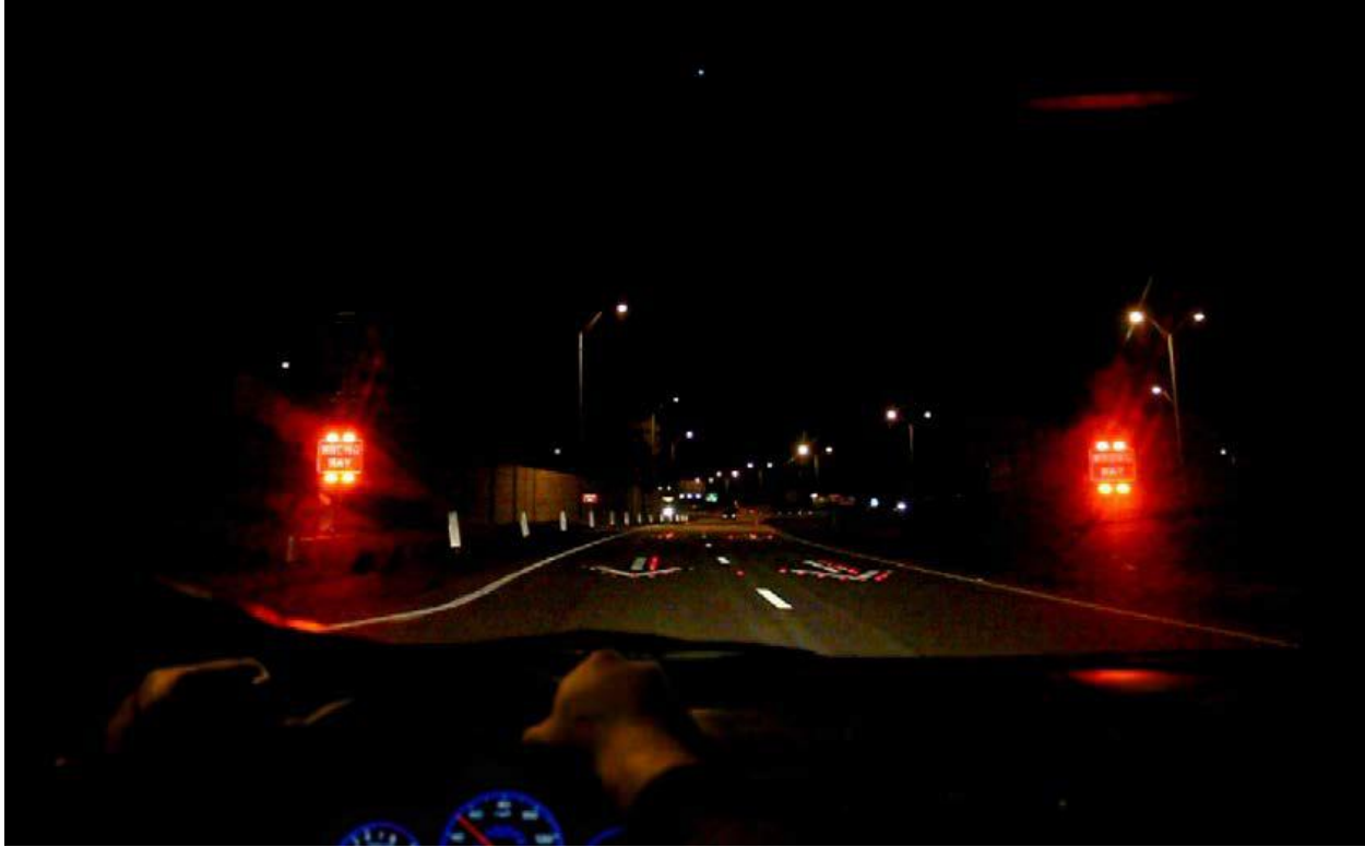
Figure 9: Red RRFBs Activated on Both Sides of Ramp
