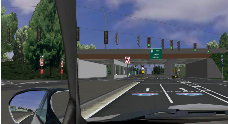
Figure E.2.3. Driving Simulator Scenario in Enhanced Countermeasure Condition, with Off-Ramp on Left
