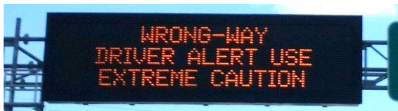
Figure 3: Wrong-way Driver Alert on Dynamic Message Sign in Florida
