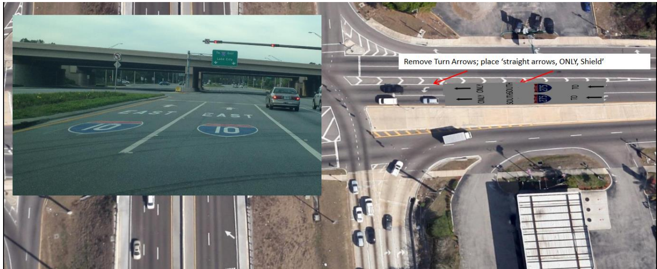
Figure 6: Newly-developed Signing and Pavement Markings (S&PM) on Arterials for Wrong-way Treatment
