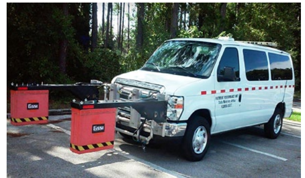
This pavement testing vehicle is equipped with ground penetrating radar.
