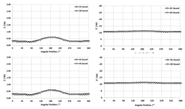
Figure B.4 Complex components of impedance, real (left) imaginary (right), for tendons #1 and #2 plotted as function of angular position for a cross-section containing Sound grout. Top and bottom: repeat measurements at ages 64 and 65 days respectively.
