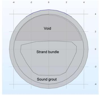
Figure 5.19 cross-sectional view of 3.5-inch nominal diameter tendon with a 4-inch long air-filled void at the center.
