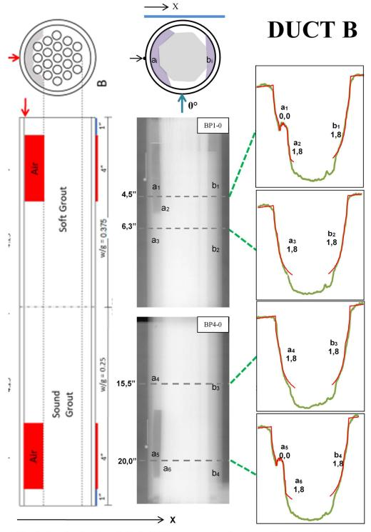
Fig. 9. Results for Duct B. Left: USF construction drawings; Center and right: Results of measurements performed by THASA, (gray indicate tendon location; purple, areas of measured grouting defects, see text).
