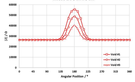
Figure 5.37 Modulus of impedance vs angular position of the tendon showing the model values for three different-size voids at 1 MHz for the profiles in Figure 5.30-5.32. The bigger the void, the higher the modulus of impedance value. The plates used for these models are 2.54 cm x 5 cm.
