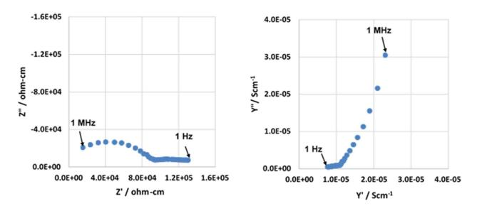
Figure A.2 Nyquist diagrams (Left: Impeditivity; Right: Admittivity) for grout in test cylinder 1a using the Wenner array test to determine impedance behavior of grout. Frequency range shown, 5 points/decade. Specimen age after casting: 193 days.
