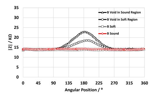
Figure 5.11 Modulus of impedance vs angular position for tendon B (age 105 days) for the different cross-sections; void in soft (P1) and void in sound grout (P4), soft (P2), and sound grout (P3).
