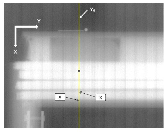
Fig. 3. Gammagraphy of a duct. The whiter horizontal bands are the strands. The X1 and X2 values indicate the pixel position along the X axis (yellow vertical line) of the edges of the strand shadow projected onto the plate. (The vertical dark lines are an instrumental defect).
