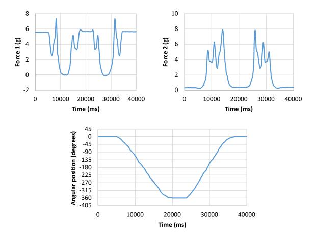
Figure 4.4 The upper two graphs show the two sensor outputs for each carriage, where Force 1 and Force 2 (in gram-force) are plotted versus time. The variation of forces as a function of position on the tendon duct perimeter reflects variations on how far the steel strand envelope is beneath each position. The lower graph shows the angular position versus time as the run is being conducted.
