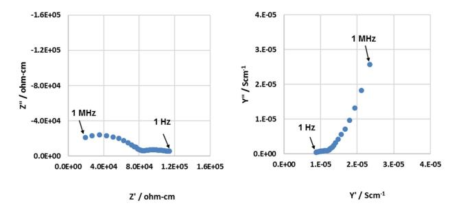
Figure A.3 Nyquist diagrams (Left: Impeditivity; Right: Admittivity) for grout in test cylinder 2b using the Wenner array test to determine impedance behavior of grout. Frequency range shown, 5 points/decade. Specimen age after casting: ~193 days.
