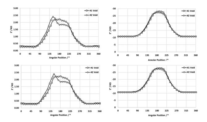
Figure B.5 Complex components of impedance, real (left) imaginary (right), for tendons #1 and #2 plotted as function of angular position for a cross-section of the central Void. Top and bottom: repeat measurements at ages 64 and 65 days respectively.
