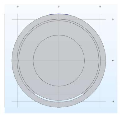
Figure 5.40 Cross-sectional view of 4-inch nominal diameter tendon with a 2-mm -thick  $(\sim73^{\circ})$  void and a 1-inch-wide plate. (Table 5.6, Tendon 3)
