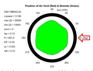
Figure 7.11 Cross-sectional image of P2-soft grout in Duct B.
