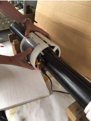
Figure 6.6 Placing the TIU-I around the tendon. Patent pending.
