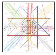
Fig. 4. Program drawing of all cones resulting from the set of X-values for every strand observed in the gammagraphies taken at different angles (shown in different colors).
