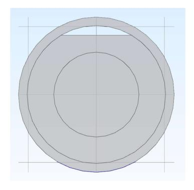
Figure 5.31 Cross-sectional view of 4-inch nominal diameter tendon, with Void #2. The plate is 5 cm x 5 cm.
