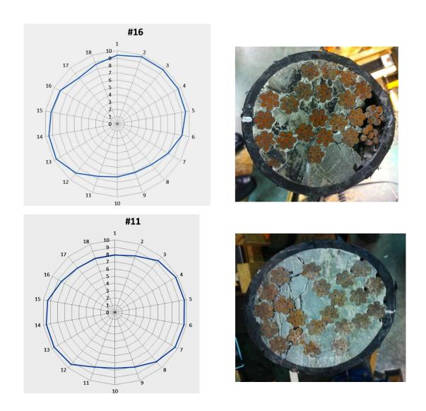
Figure 4.8 Results of semiquantitative strand configuration evaluation using an inductance device applied to two tendon samples from the John Ringling Causeway Bridge.
