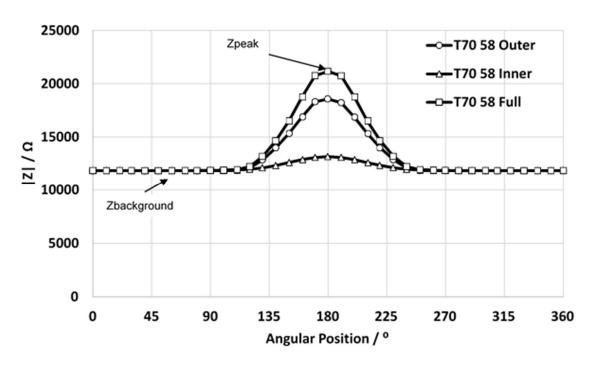
Figure 5.33 Modulus of impedance vs. angular position of the tendon showing the model values for a full, outer and inner void at 1 MHz for the profiles in Figure 5.24-5.26. The plates used for these models are 5 cm x 5cm.
