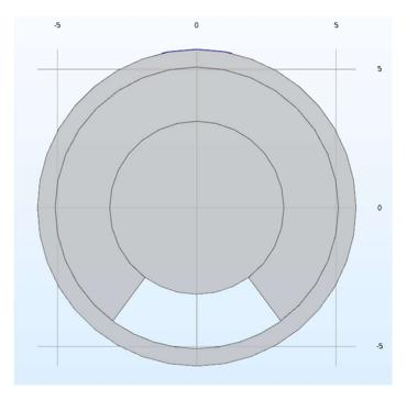
Figure 5.38 Cross-sectional view of 4-inch nominal diameter tendon with a Full ~73° void and a 1 inch wide plate. (Table 5.6, Tendon 1)
