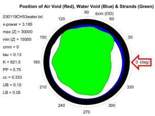
Figure 7.19 Cross-sectional image of P5-water void (after adding water) in Duct C. The TIU-II captured the 3"-long ½" bolt.
