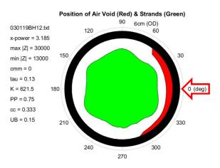
Figure 7.10 Cross-sectional image of P1-air void in Duct B.
