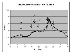
Fig. 6. Gammagraphy of a severe void in a PT duct and its quantitative determination.
