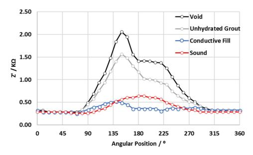
Figure 5.6 Real part of the complex impedance vs. angular position for Tendon #2 (age 166 days for void and sound, 163 days for unhydrated grout, and 169 days for conductive fill) at center with section filled with air, unhydrated grout, and conductive fill. Impedance results for a sound cross-section also included. All experimental results in this and subsequent figures are for a frequency of 1 MHz.
