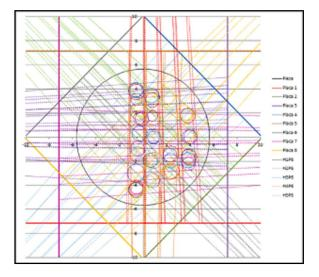
Fig. 5. Program drawing of all cones and intersections defining strands (case of Duct A).
