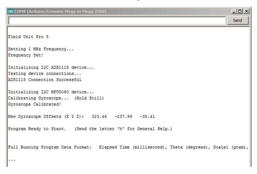
Figure 6.5 Screenshot of serial monitor after the TIU-I has calibrated and is ready to obtain an IA pending commands from the operator.
