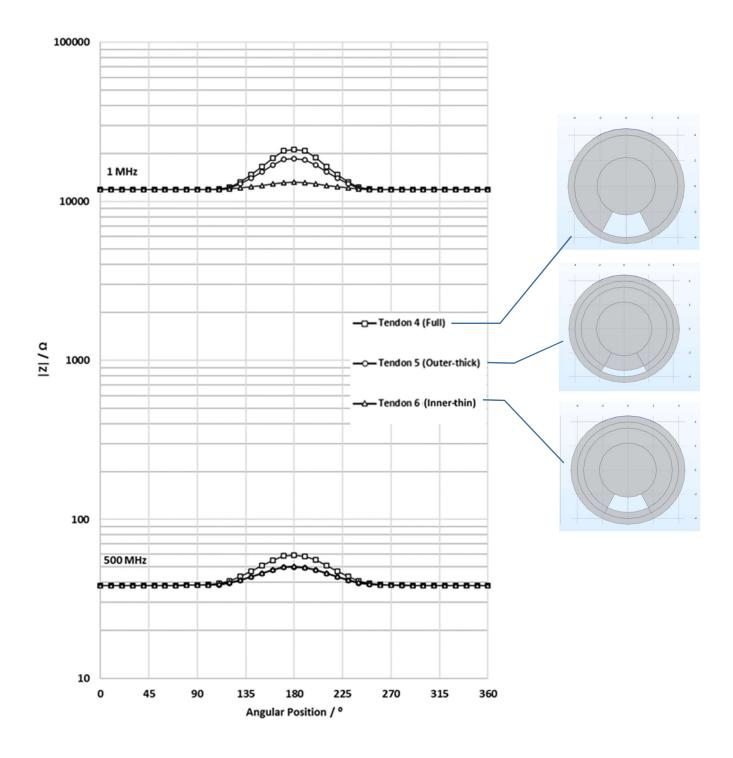
Figure 5.42 Modulus of impedance vs. angular position for Table 5.6; Tendons 4, 5, and 6 at 1 MHz and 500 MHz. Log scale y-axis permits direct comparison of relative descriptors. Note that at 1 MHz, the outer void is strongly apparent, but the inner void is barely detectable. Using 500 MHz instead, the results can identify the void regardless of whether it is on the outer part of the cross-section or buried deeper.
