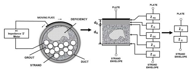
Figure 5.1 Left: Electromagnetic coupling test method arrangement. The moving metal plate is shaped to fit the external duct surface. Center: Simplified composite dielectric/conductive configuration. Right: Further simplification
