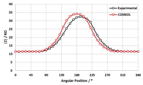
Figure 5.23 Modulus of impedance vs. angular position of the tendon (with air void) showing the experimental values (from Figure 5.9) and the model values at 1 MHz for the profile in Figure 5.19. The model results follow the experimental trends.
