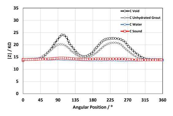
Figure 5.12 Modulus of impedance vs angular position for tendon C (age 105 days) for the different cross-section; void (P3), unhydrated grout (P1), water (P5), and sound grout (P2).
