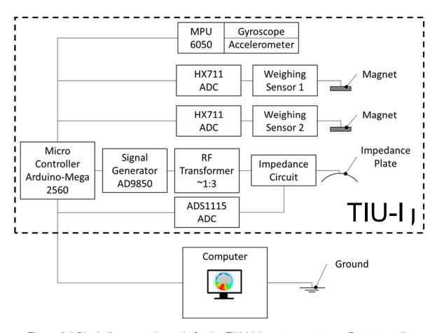
Figure 6.1 Block diagram schematic for the TIU-I laboratory prototype. Patent pending.
