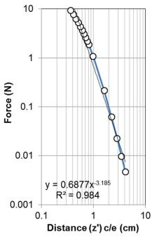
Figure 4.11 Model results of Force (N) vs. z', the center-to-edge distance between the magnet and the steel rod, the trendline is a nominal abstraction roughly indicative of characteristic response in the interval examined.
