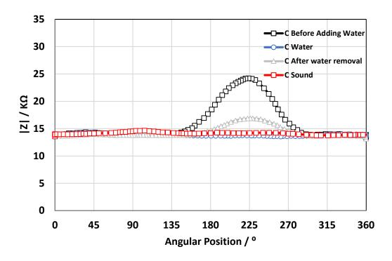
Figure 5.13 Modulus of impedance vs angular position for tendon C (age 105 days) for the same void (P5) before adding water, when water was added, and ~30 min after the water was removed. Impedance results for a sound cross-section also
