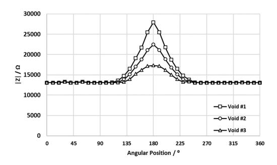
Figure 5.36 Modulus of impedance vs. angular position of the tendon showing the model values for three different-size voids at 1 MHz for the profiles in Figure 5.30-5.32. The bigger the void, the higher the modulus of impedance value. The plates used for these models are 5 cm x 5 cm.
