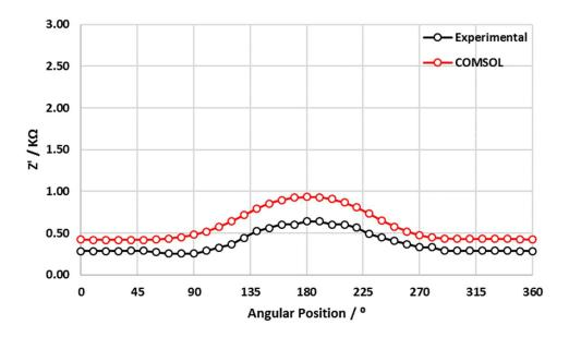
Figure 5.20 Real impedance value vs. angular position of the tendon (sound grout) showing the experimental values (from Figure 5.6) and the model values at 1 MHz for the profile in Figure 5.18. The model results follow the experimental trends.
