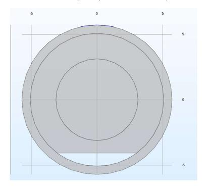
Figure 5.39 Cross-sectional view of 4-inch nominal diameter tendon with Void #1(~73°) and a 1 inch wide plate. (Table 5.6, Tendon 2)
