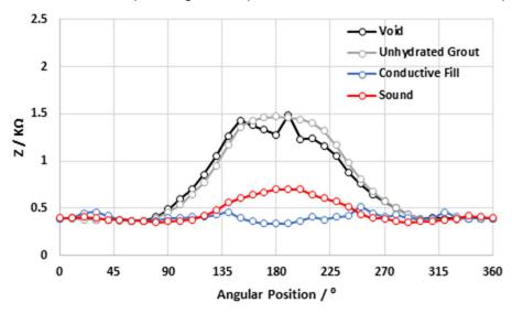
Figure B.1 Real part of the complex impedance vs. angular position for Tendon #1 (age 705 days) at center with section filled with air, unhydrated grout, and conductive fill. Impedance results for a sound cross-section also included.
