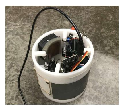
Figure 6.4 TIU-I placed in the vertical calibration position away from steel mass. Patent Pending.
