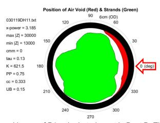
Figure 7.20 Cross-sectional image of P1-unhydrated grout in Duct D. The TIU-II did not capture the internal void.
