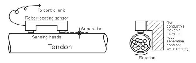
Figure 4.7 Schematic of the Model C-4956 R-Meter® placement.
