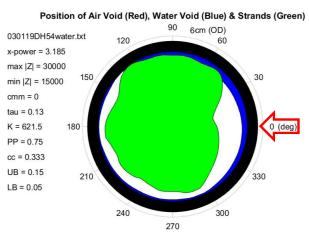
Figure 7.25 Cross-sectional image of P5-air void (after adding water) in Duct D.
