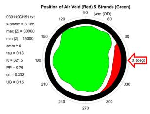
Figure 7.18 Cross-sectional image of P5-air void (before adding water) in Duct C. The TIU-II captured the 3"-long ½" bolt.
