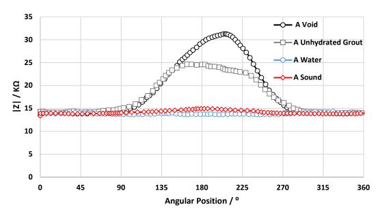
Figure 5.10 Modulus of impedance vs angular position for tendon A (age 105 days) for void (Position P3), unhydrated grout (P1), water (P5), and sound cross-section (P2).
