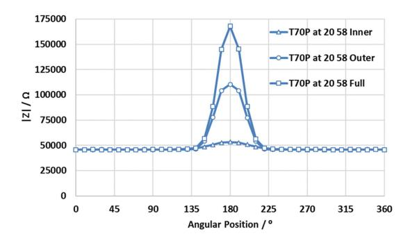
Figure 5.35 Modulus of impedance vs. angular position of the tendon showing the model values for a full, outer, and inner void at 1 MHz for the profiles in Figure 5.24-5.26. The plates used are guarded.
