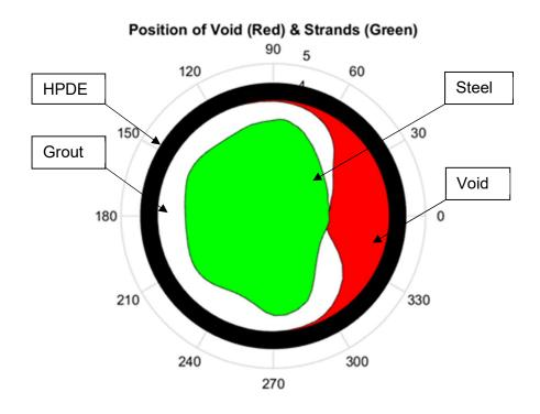
Figure 6.3 Image generated from the TIU-I after scanning an in-house cast tendon with the device centered on an existing void. Patent pending.
