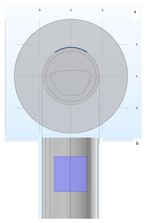
Figure 5.17 (a) – Cross-sectional view of 3.5-inch (8.9-cm) nominal outer diameter tendon with steel strand envelope imported from steel strand location detector prototype. The tendon is surrounded by a 9-cm radius air cylinder to represent field and laboratory conditions. (b)— Top view of 5 cm x 5 cm plate used for model (edge view on (a)). Grid scale is in cm.
