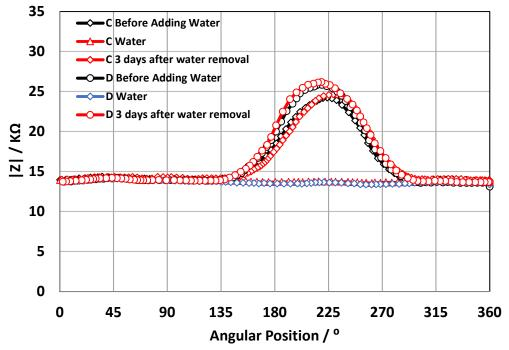
Figure 5.16 Modulus of impedance vs angular position for tendons C and D (age 105 days) for the same void (P5) before adding water, when water was added, and 3 days after the water was removed.
