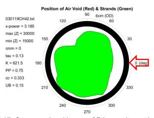
Figure 7.17 Cross-sectional image of P4-sound grout in Duct C.
