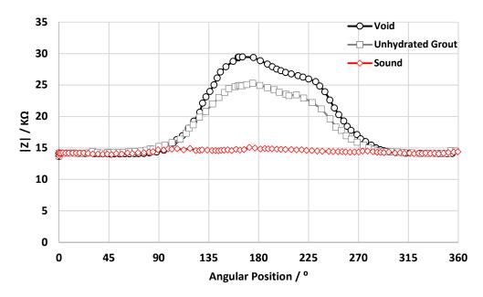
Figure 5.9 Modulus of impedance vs angular position for tendon A, at the same void (Position P1) that had air (age 36 days) and then was filled with unhydrated grout (age 55 days). Impedance results for a sound cross-section (P2) (age 55 days) also included. All experimental results in this and subsequent figures are for a frequency of 1 MHz.
