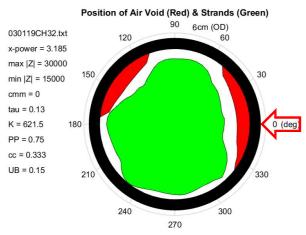
Figure 7.16 Cross-sectional image of P3-air void in Duct C.
