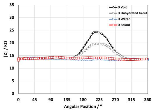
Figure 5.14 Modulus of impedance vs angular position for tendon D (age 105 days) for the different cross-section; void (P3), unhydrated grout (P1), water (P5), and sound grout (P2).
