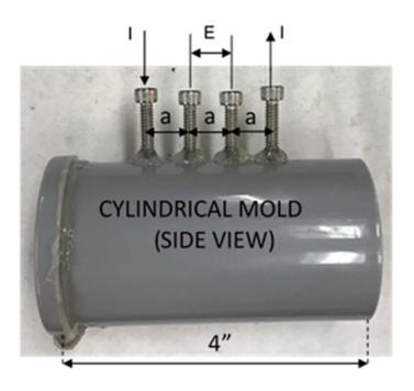
Figure A.1 Top and side view of cylindrical mold used for EIS, resistivity Wenner array test.
