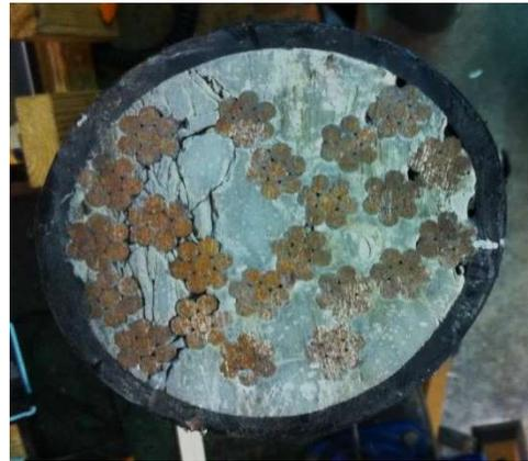
Figure 4.8 Results of semiquantitative strand configuration evaluation using an inductance device applied to two tendon samples from the John Ringling Causeway Bridge.
