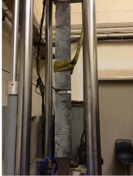
Figure 2-17: Specimen 2 failure in tension
