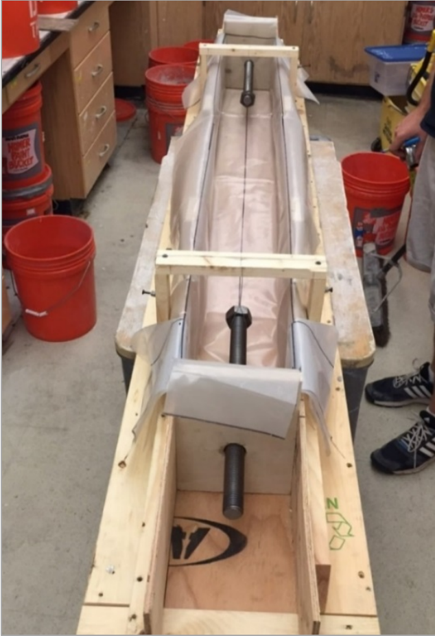
Figure 2-3: Wooden forms for 6” x 6” x 60” concrete specimen
