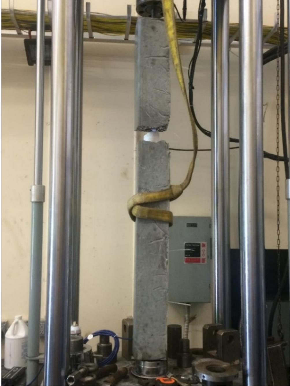
Figure 2-6: Concrete specimen 1 fractured in tension
