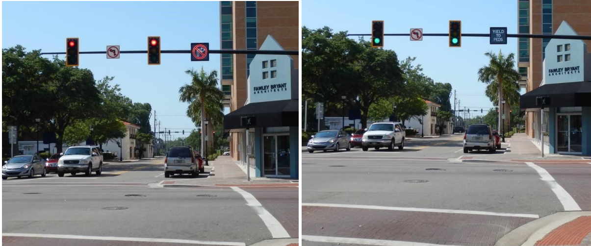
Figure D-1 LPI with dual blank-out sign in Bradenton.
