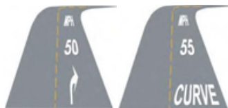
Figure 43. Advanced Pavement Markings for Curve Warning and Advisory Speed
