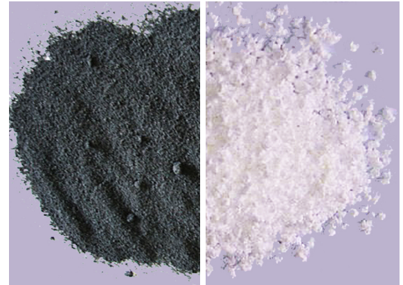
Ground tire rubber (GTR; left) and styrene butadiene styrene (SBS; right) are frequently used as asphalt additives.
