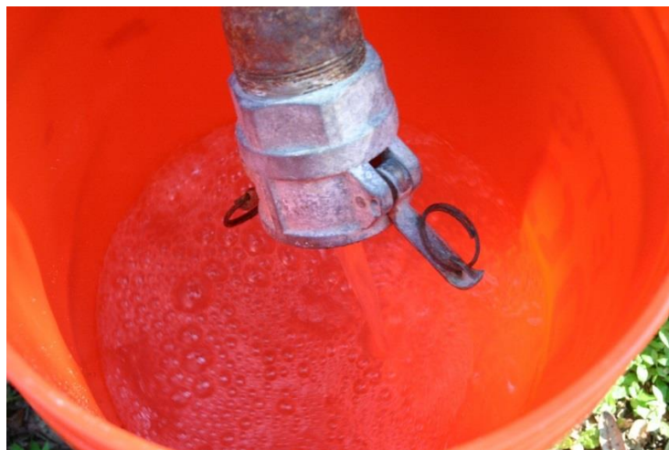
Figure 3.60 Gravity feed of KB International Enhanced CDP polymer into 5 gallon bucket.
