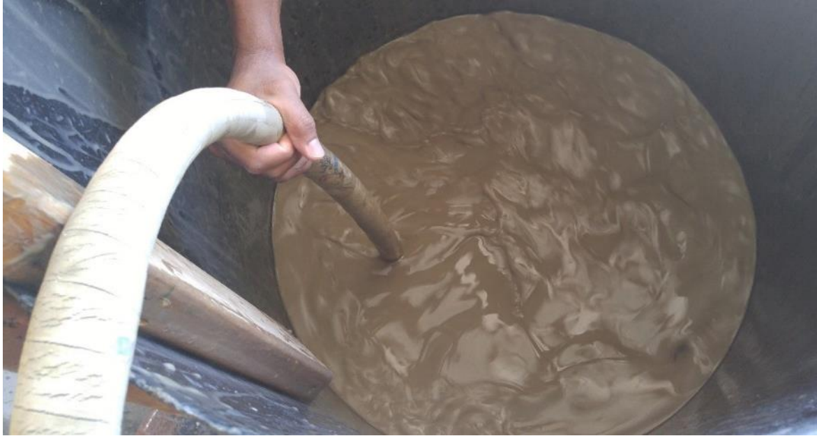
Figure 3.27 Slurry in the mixing tank.
