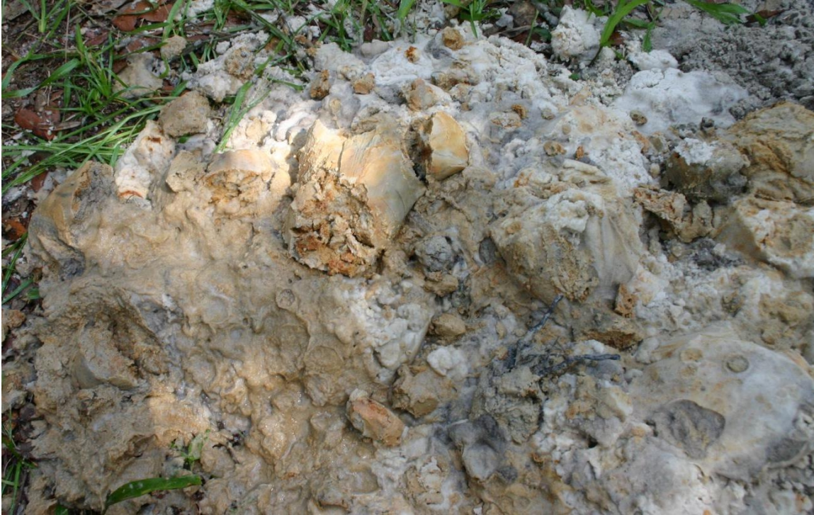
Figure 3.64 Clayey-sand encountered during excavation of KB5-1hr borehole.
