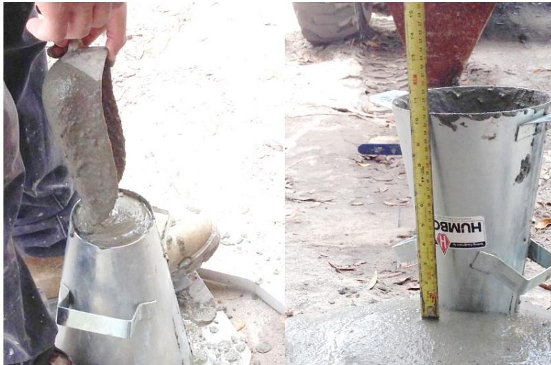
Figure 3.34 Filling the slump cone (left), measuring the slump of 10.5in (right).
