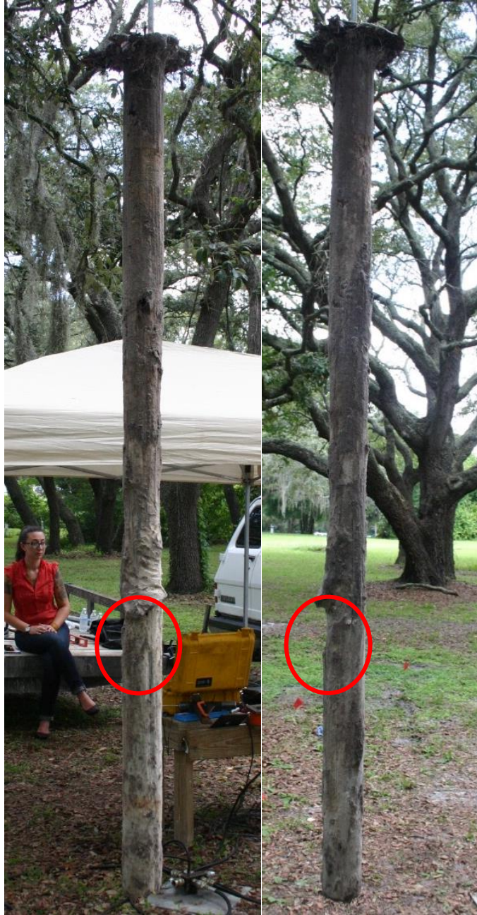
Figure 3.67 Anomaly encountered on KB2-8hr shaft.
