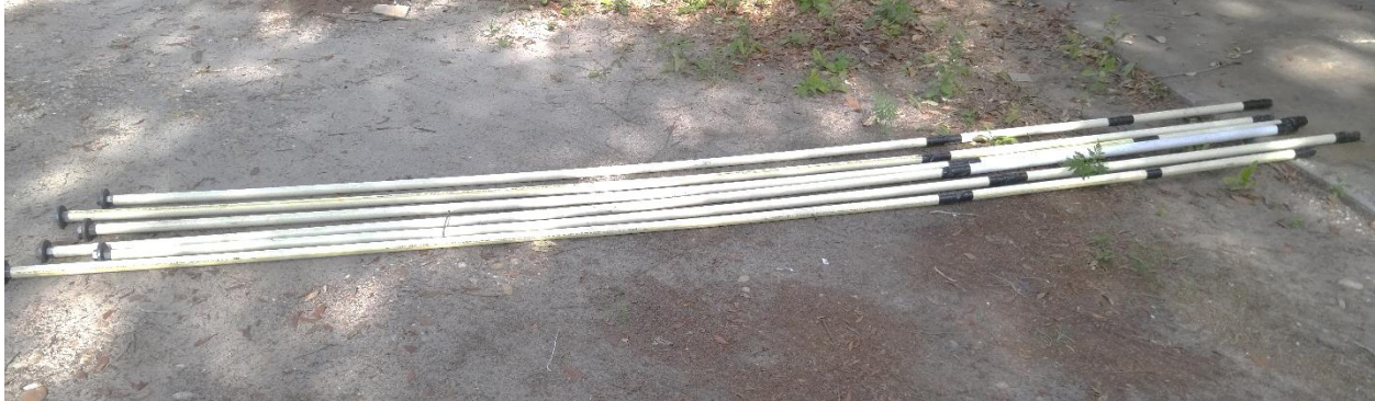
Figure 3.11 Sheathed \frac{3}{4} in all-thread steel bar.
