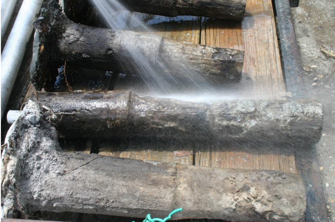
Figure 3.72 Soil bonded to concrete surface in upper 3ft of KB Polymer shafts.
