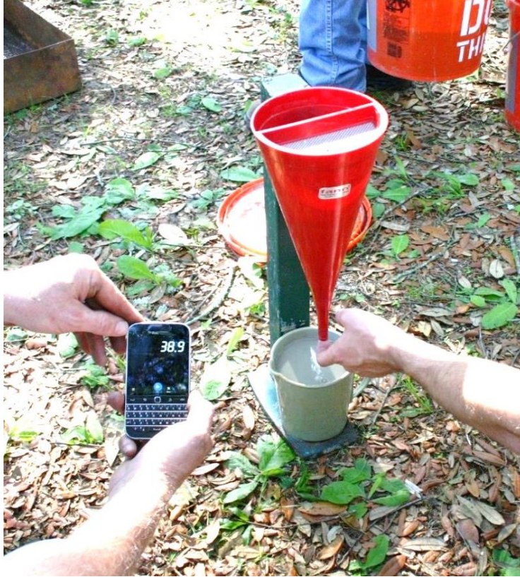
Figure 3.44. Marsh funnel viscosity field test.
