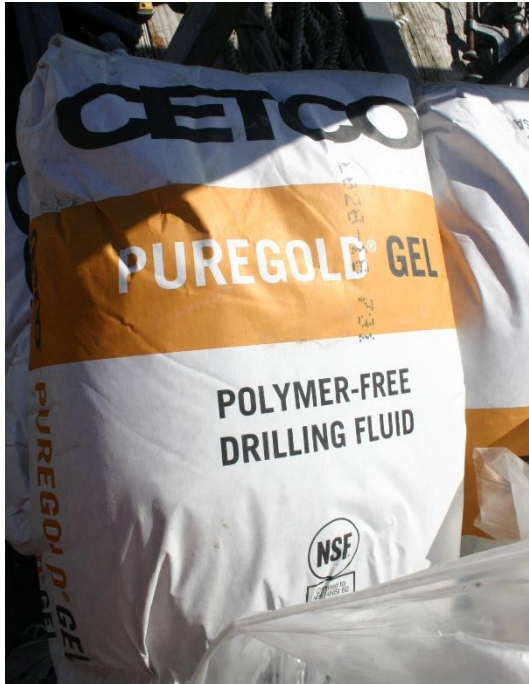
Figure 4.7 Slurry products used: CETCO Puregold Gel bentonite (left); Matrix Big Foot polymer (right).
