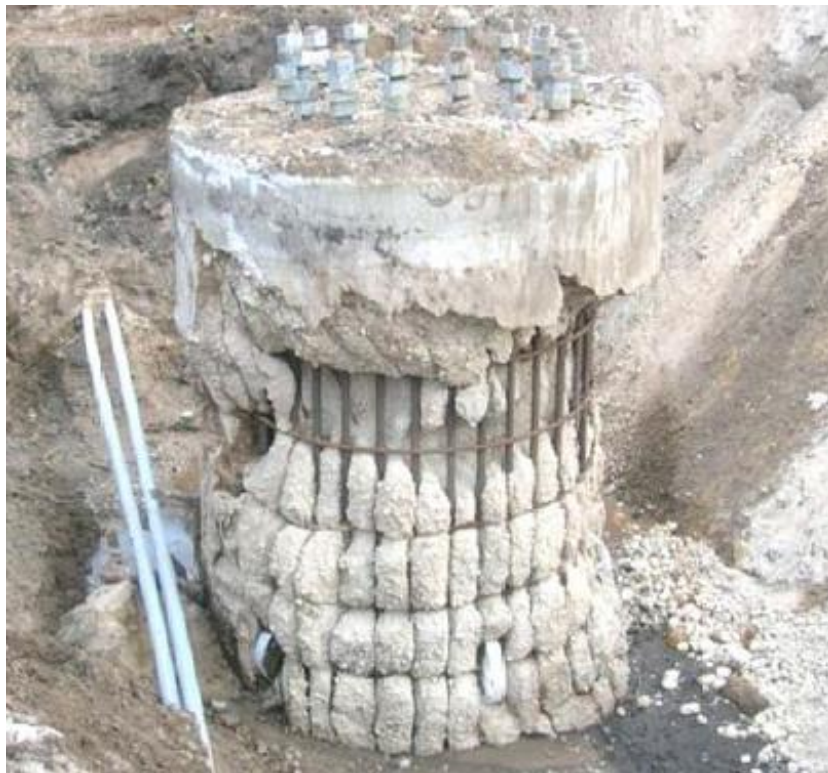
Figure 2.5 exhumed shaft showing poor concrete flow resulting from poor slurry/concrete properties (Mullins et al., 2014).
