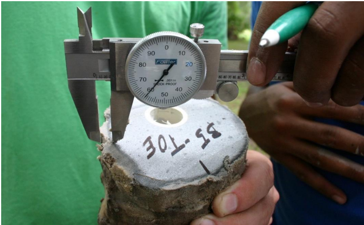
Figure 3.57 Measurement of bentonite filter cake thickness.
