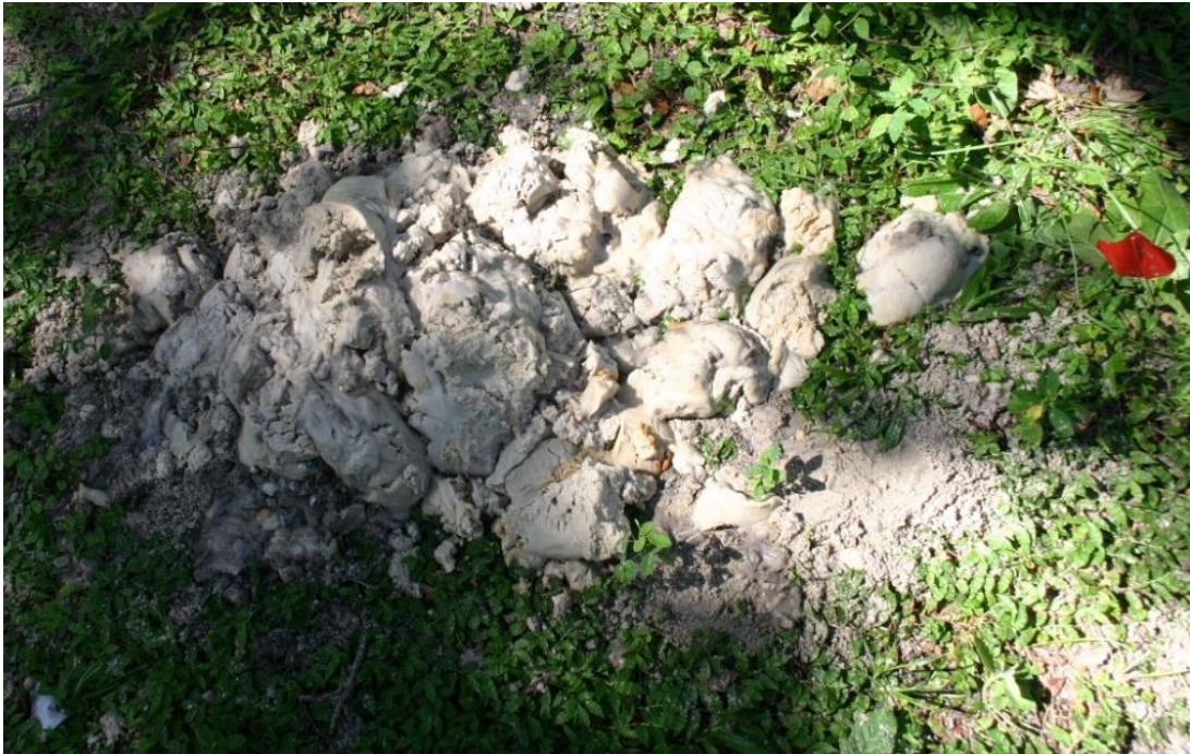
Figure 3.75 Soil excavated with Matrix Bigfoot polymer.
