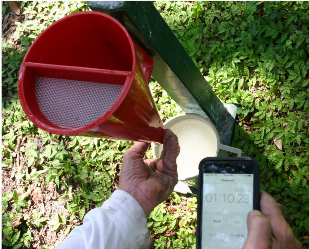
Figure 3.76 Matrix Bigfoot polymer field Marsh funnel test (70sec/qt).
