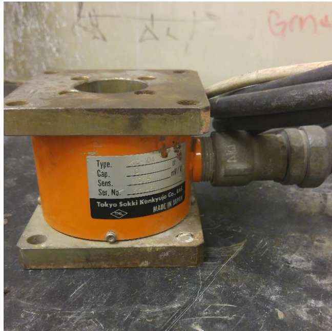
Figure 3.24 Compression type load cell (10 ton).
