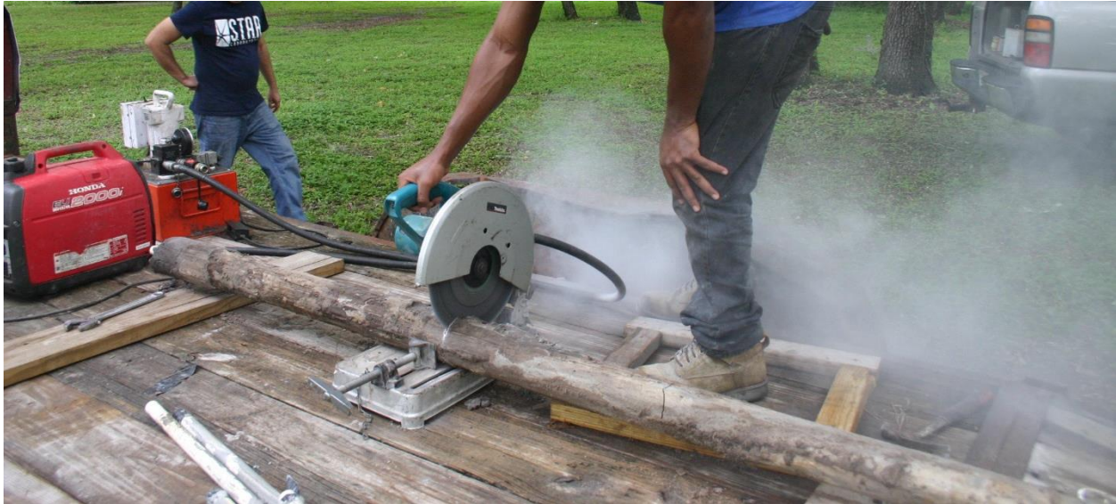
Figure 3.56 Cutting of shafts at quarter points.
