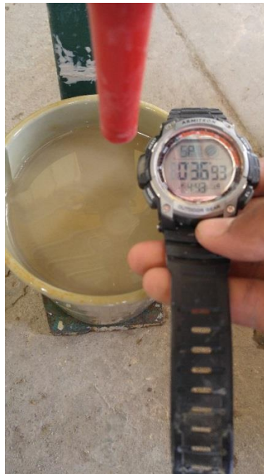
Figure 3.28 Marsh funnel viscosity at time of drilling (37s/qt).
