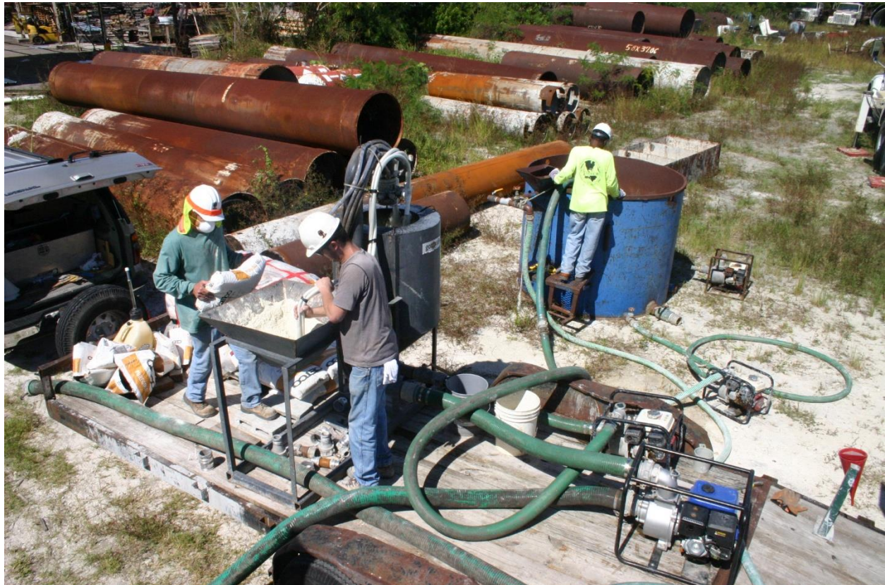
Figure 4.8 Multi-educator mixing system used to prepare slurry.
