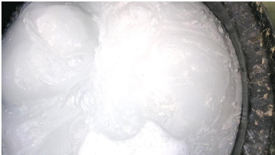
Figure 3.33 Mixing of Cetco polymer stabilizing system.
