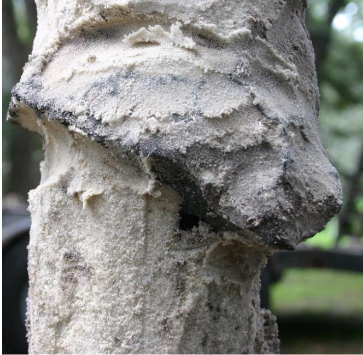
Figure 3.68 Close up of anomaly encountered on KB2-8hr shaft.
