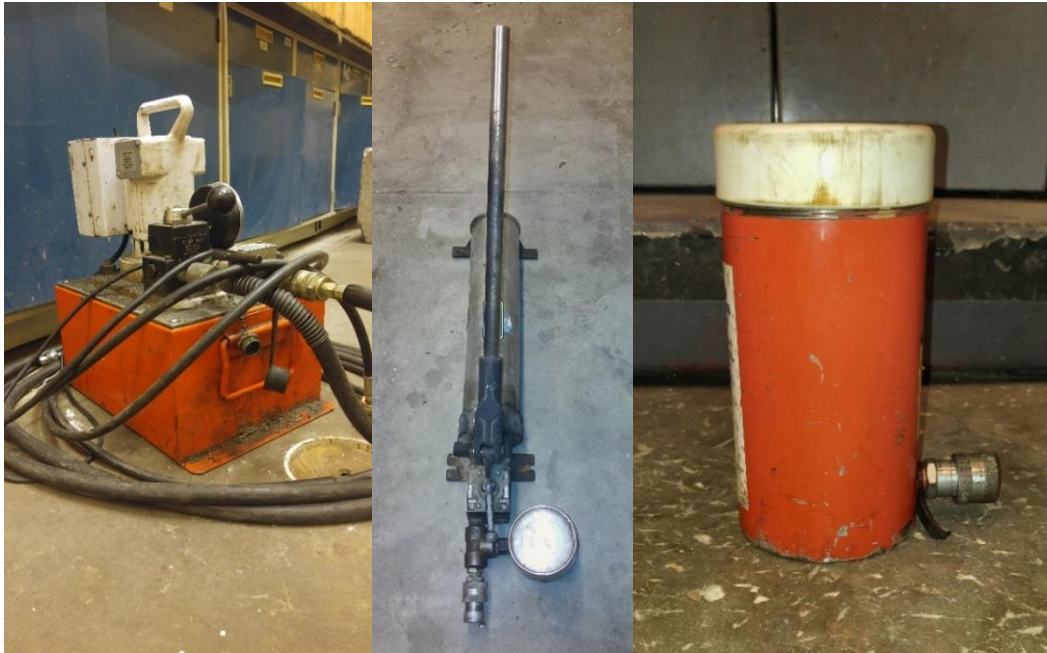
Figure 3.21 Electric hydraulic pump (left), hand hydraulic pump (middle), hydraulic ram (right).
