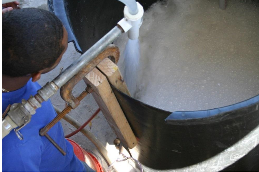
Figure 3.7 Hootonanny™ discharging product into mixing tank.
