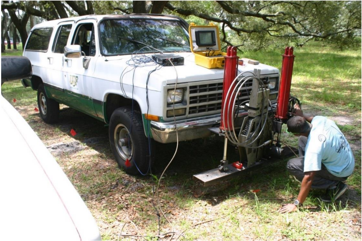
Figure 3.2 Cone Penetration Testing.
