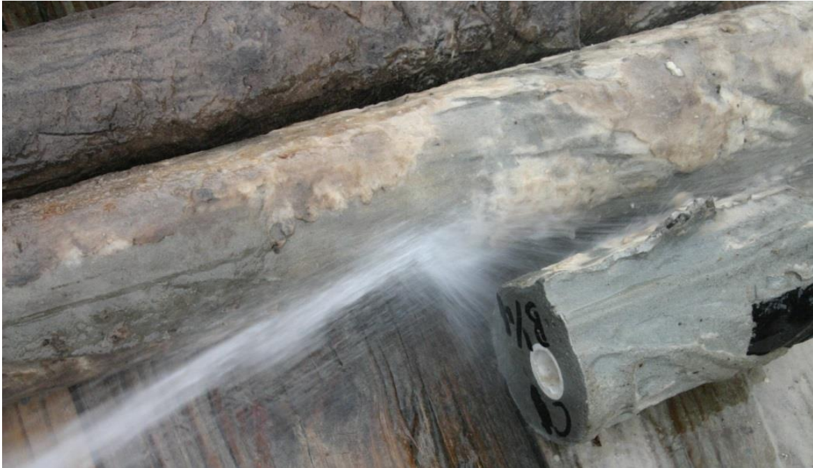
Figure 3.91 Removal of soil cake on Cetco polymer shafts.
