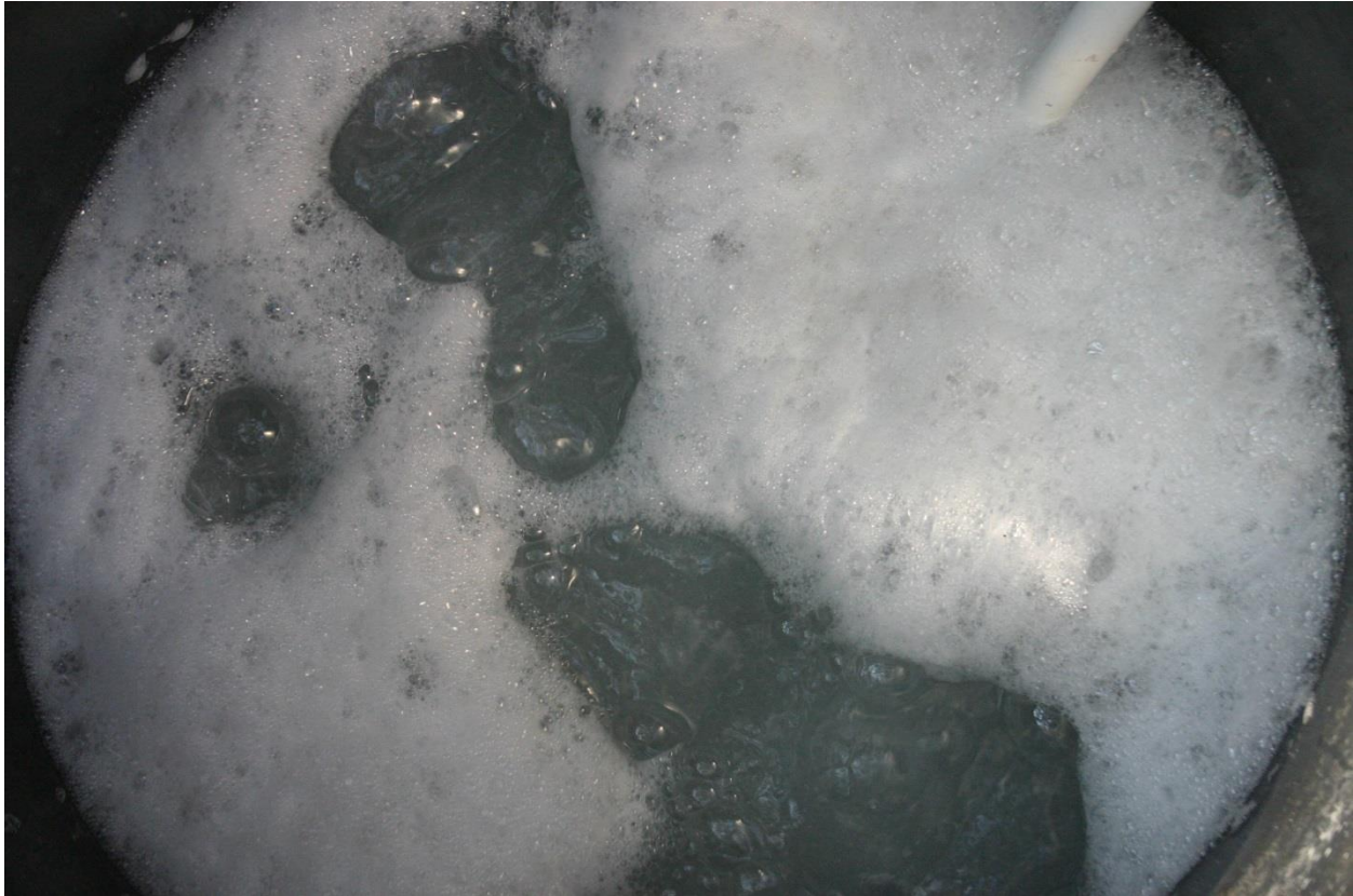
Figure 3.30 Continuous agitation of KB International Enhanced CDP polymer with aerator.
