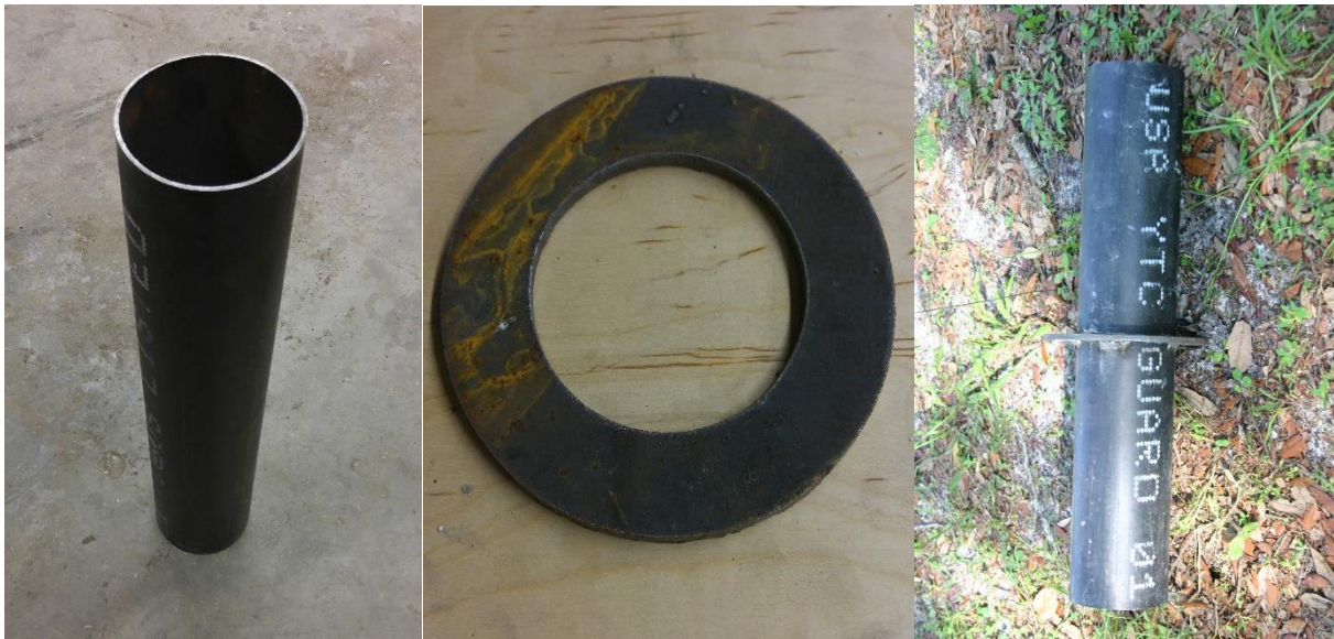
Figure 3.6 casing tubing (left), casing ring (middle) & assembled casing (right).
