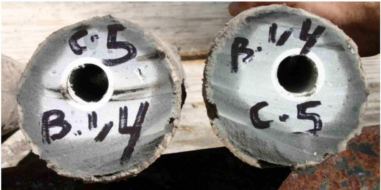
Figure 3.90 Dissected cross section of Cetco polymer shaft.
