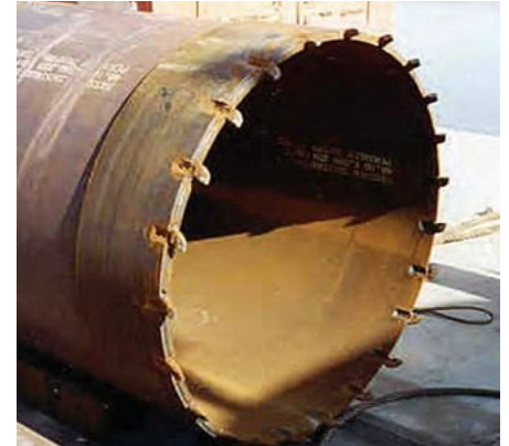
This casing is equipped with cutting teeth to help it drill into rock layers.
