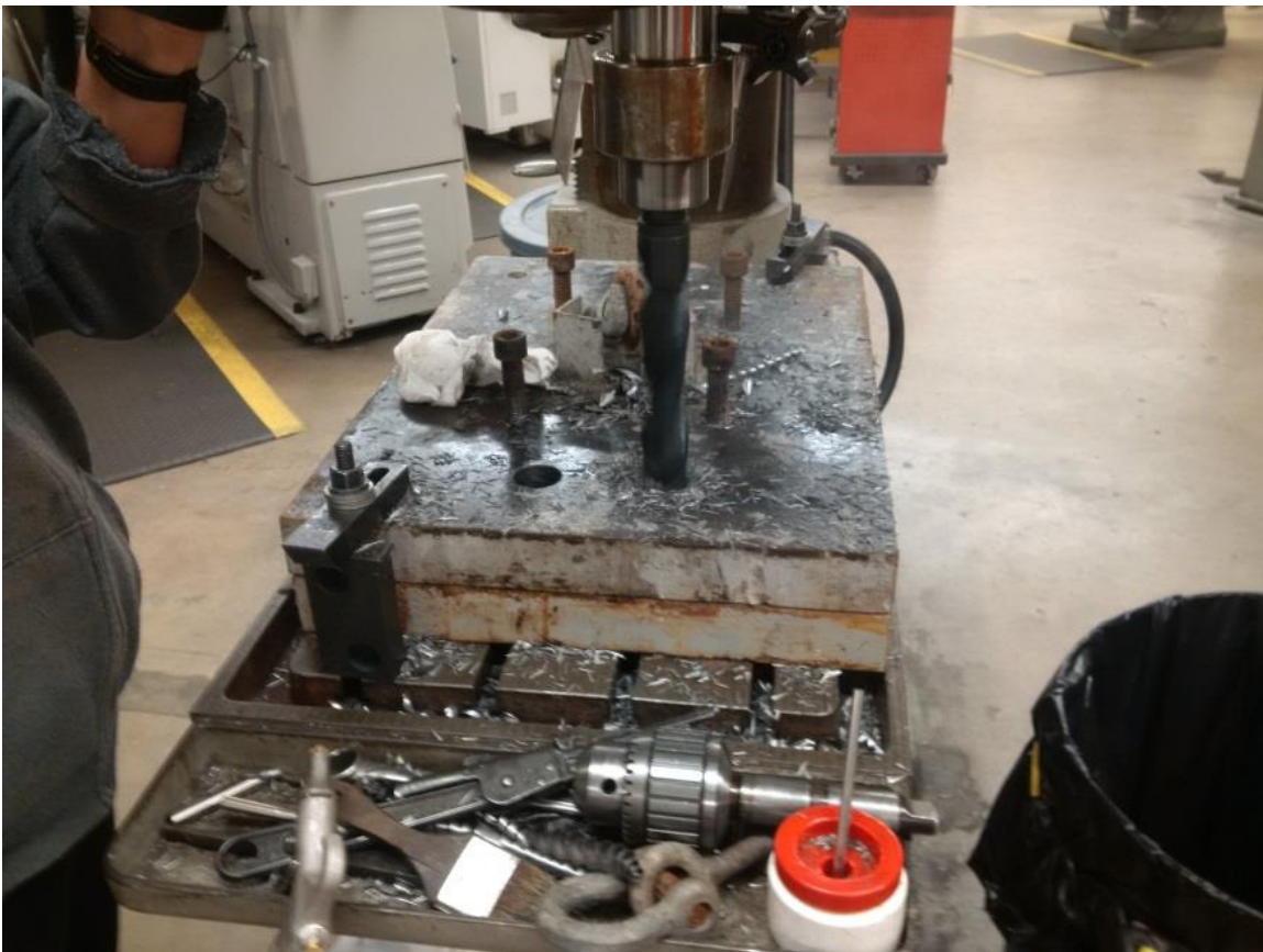
Figure 4.15 Two 18in x 24in x 2in thick plates match drilled as top load transfer beam.
