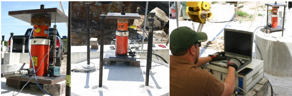
Figure 3.18 Pull-out load test in progress.
