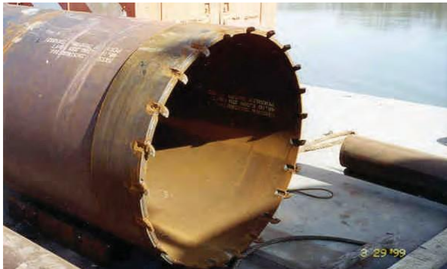
Figure 2.11 Cutting Teeth on the Casing to Assist Penetration into the Bearing Stratum (FHWA, 2010).
