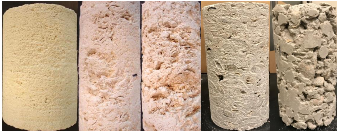
Figure 3.1 Field retrieved limestone cores (left); core from simulated limestone bed and simulated limestone cylinder specimen (right).
