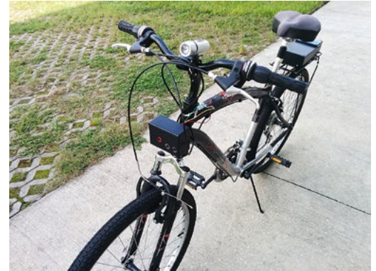
The BDAS' black boxes, mounted on the front and rear of this bicycle, contain sensors and cameras.
