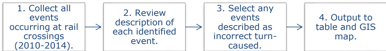
Figure 2-2 Procedure to filter events caused by incorrect turns at highway-rail grade crossings from the FRA database.
