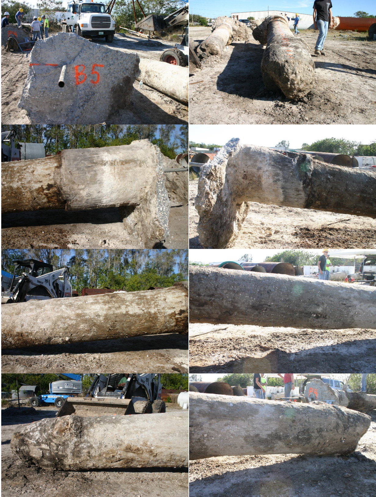
Figure B.7. Shaft B-5 (from top to bottom): shaft top (left) and toe (right); side views of shaft top section; side views of shaft middle section; side views of bottom section
