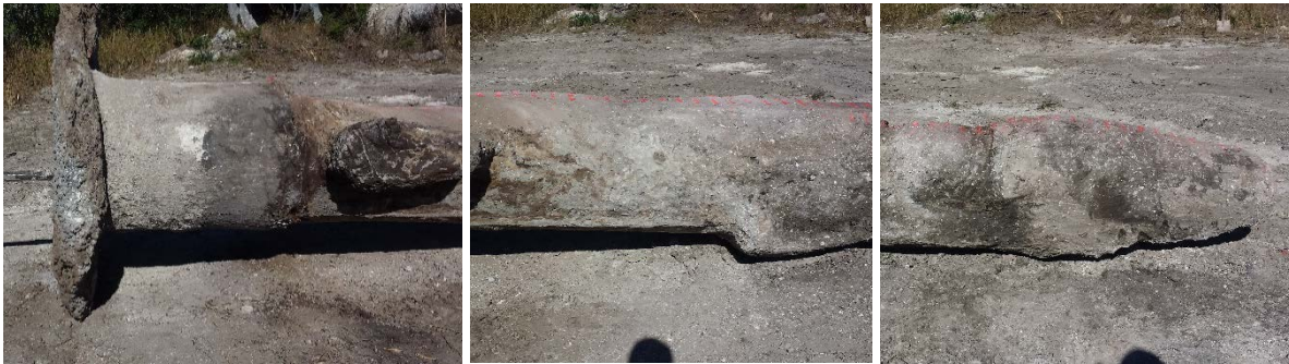
Figure 5.7. Top, middle, and bottom (left to right) of exhumed shaft P5
