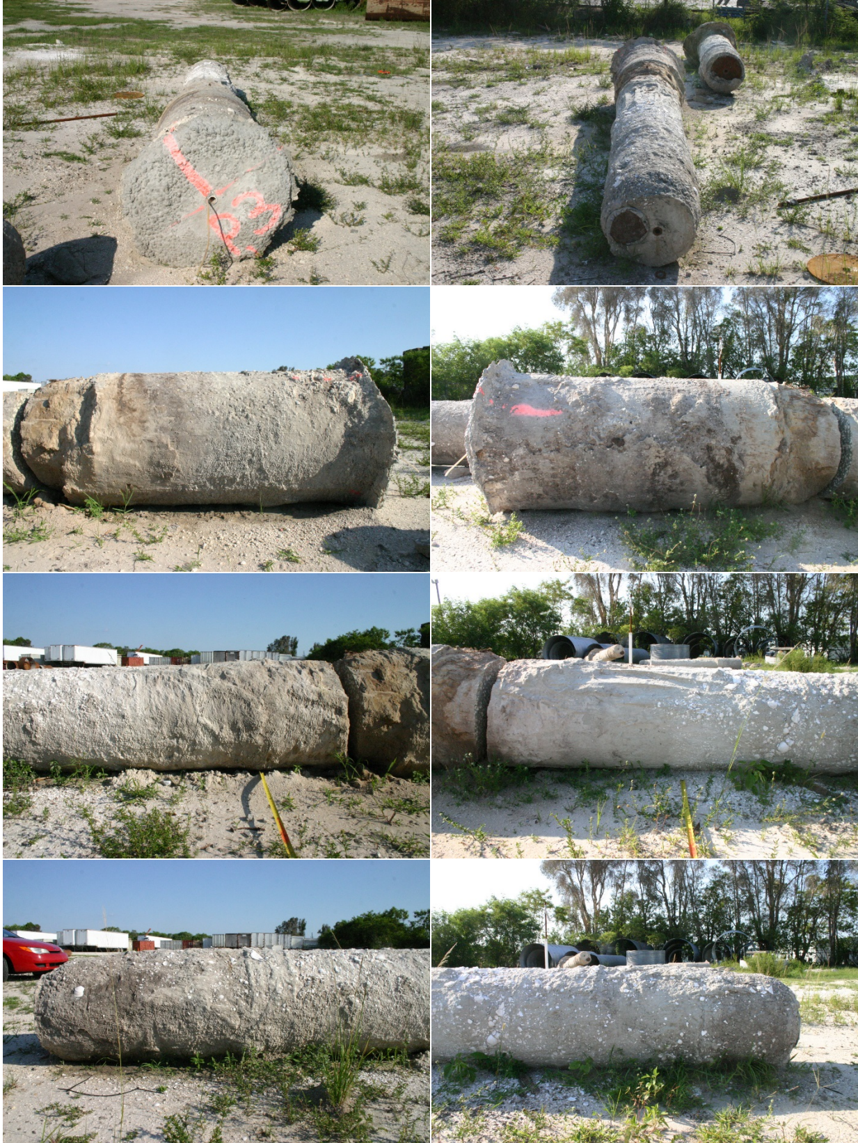
Figure B.3. Shaft P-3 (from top to bottom): shaft top (left) and toe (right); side views of shaft top section; side views of shaft middle section; side views of bottom section
