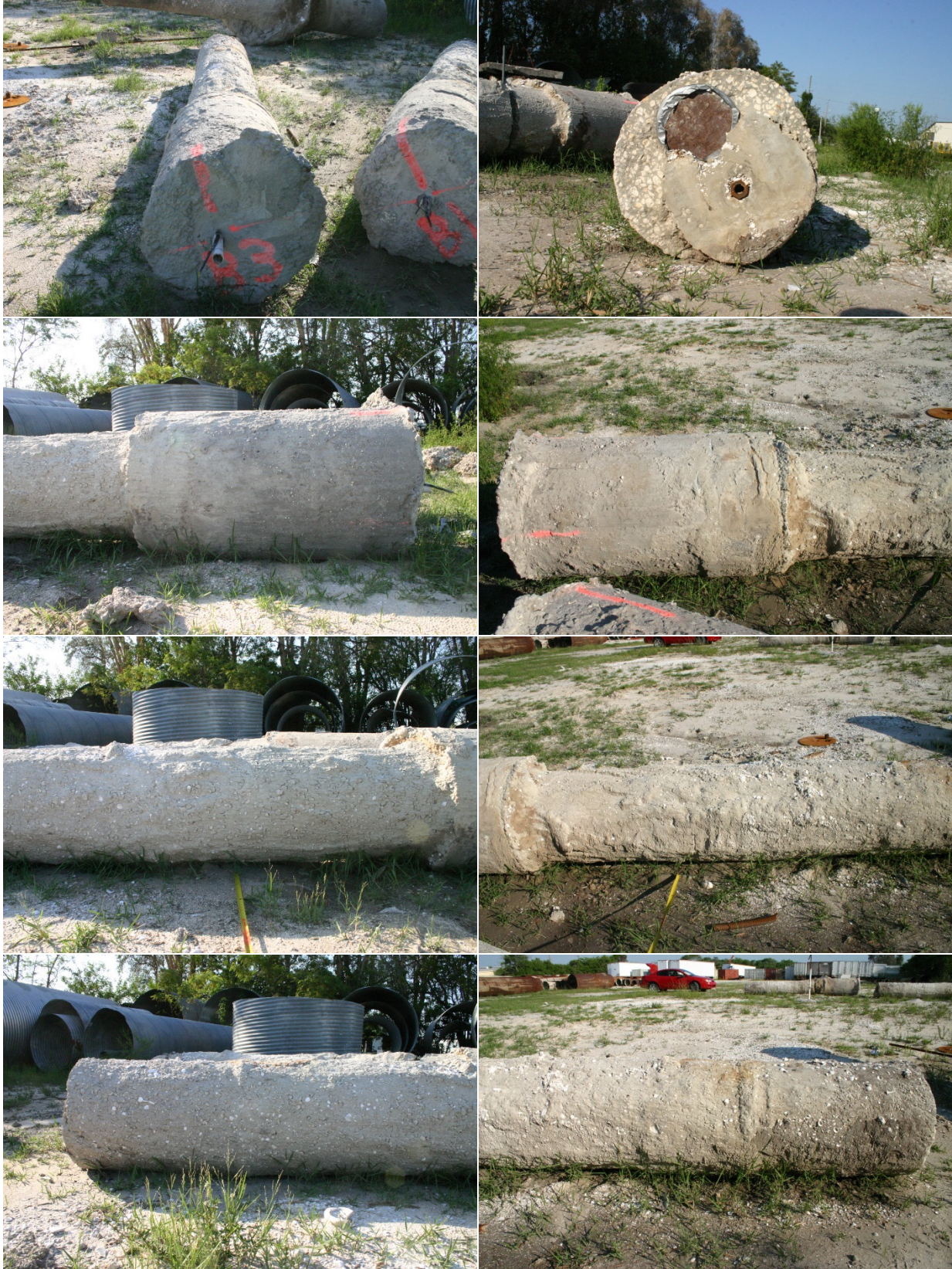
Figure B.4. Shaft B-3 (from top to bottom): shaft top (left) and toe (right); side views of shaft top section; side views of shaft middle section; side views of bottom section
