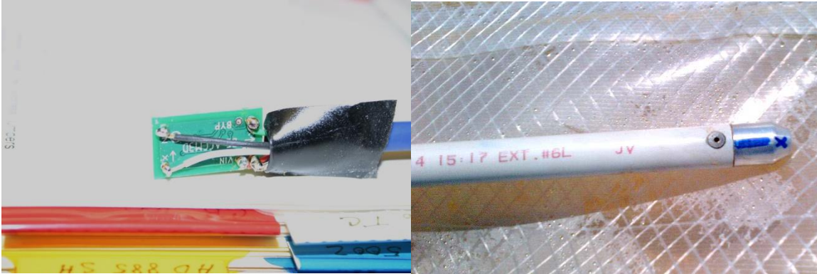
Figure 4.5. Circuit board installed in PVC delivery rod
