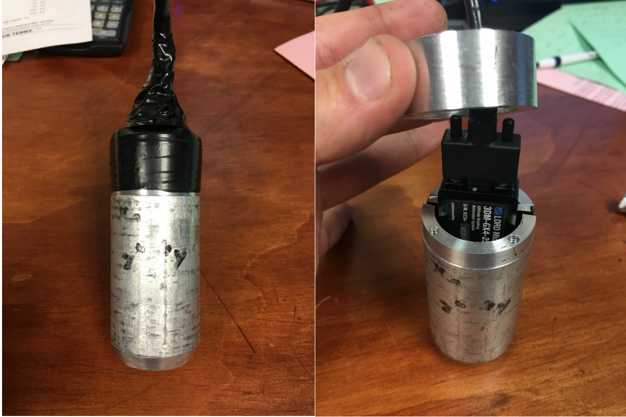
Figure 4.22. Aluminum probe body with housed IMU sensor
