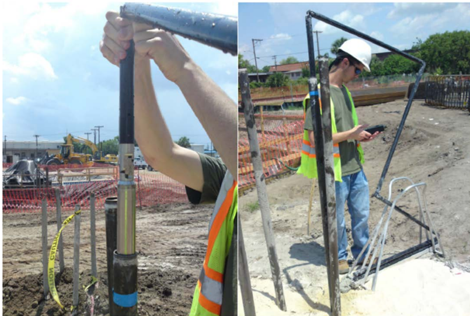
Figure 4.1. Groove-less casing with wheel-less inclinometer
