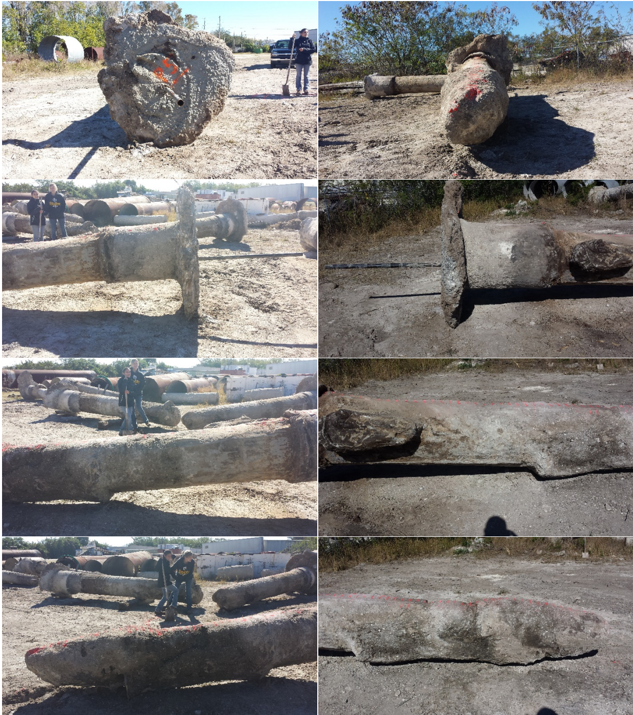
Figure B.9. Shaft P-5 (from top to bottom): shaft top (left) and toe (right); side views of shaft top section; side views of shaft middle section; side views of bottom section
