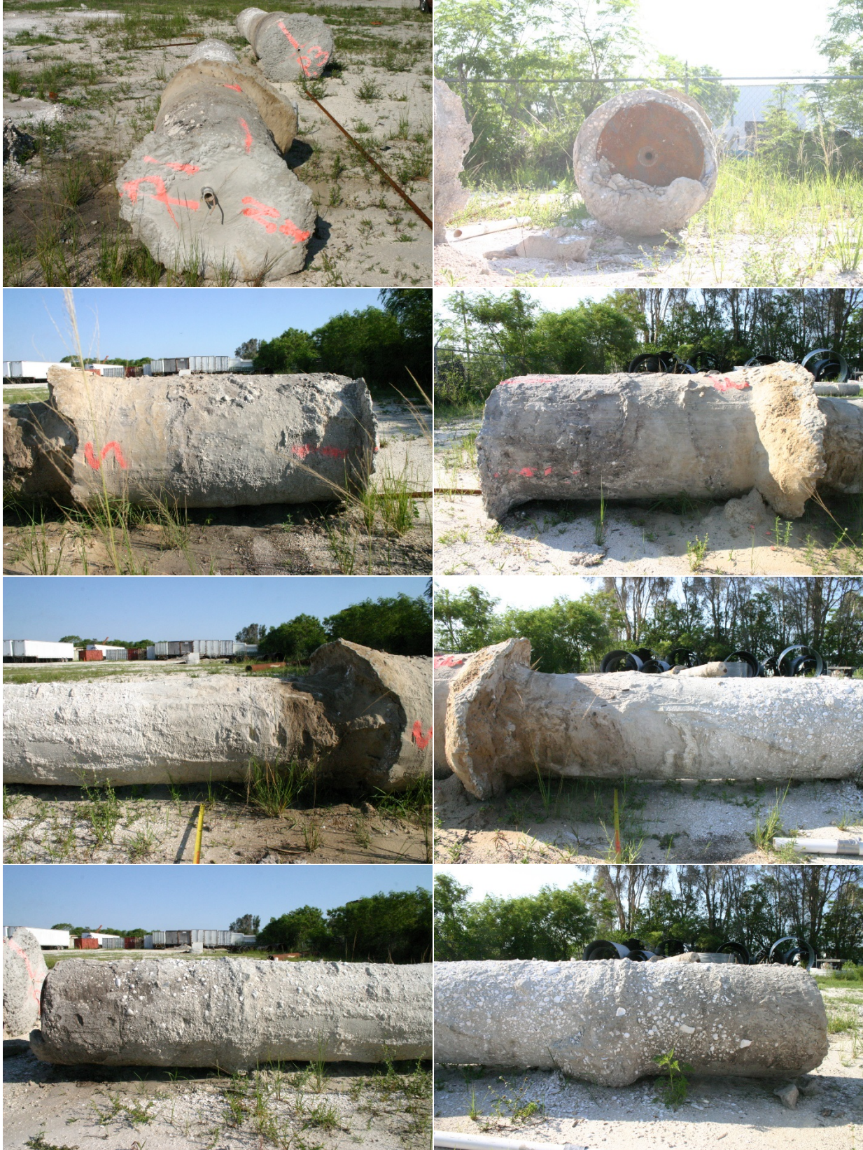
Figure B.2. Shaft P-1 (from top to bottom): shaft top (left) and toe (right); side views of shaft top section; side views of shaft middle section; side views of bottom section
