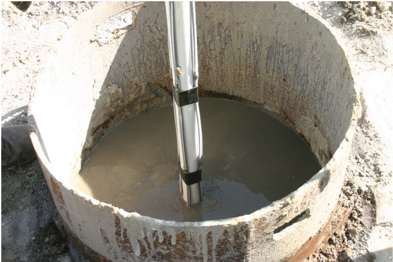
Figure 5.8. 1.5in PVC instrumented with four orthogonal thermal wires placed in center of shaft
