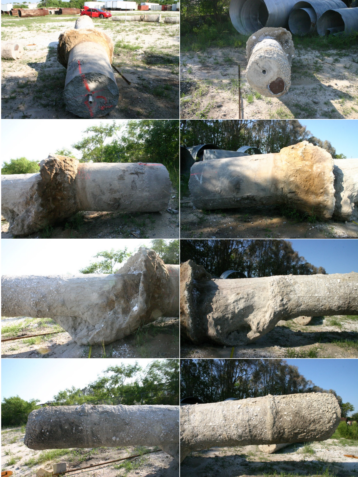
Figure B.5. Shaft P-2 (from top to bottom): shaft top (left) and toe (right); side views of shaft top section; side views of shaft middle section; side views of bottom section
