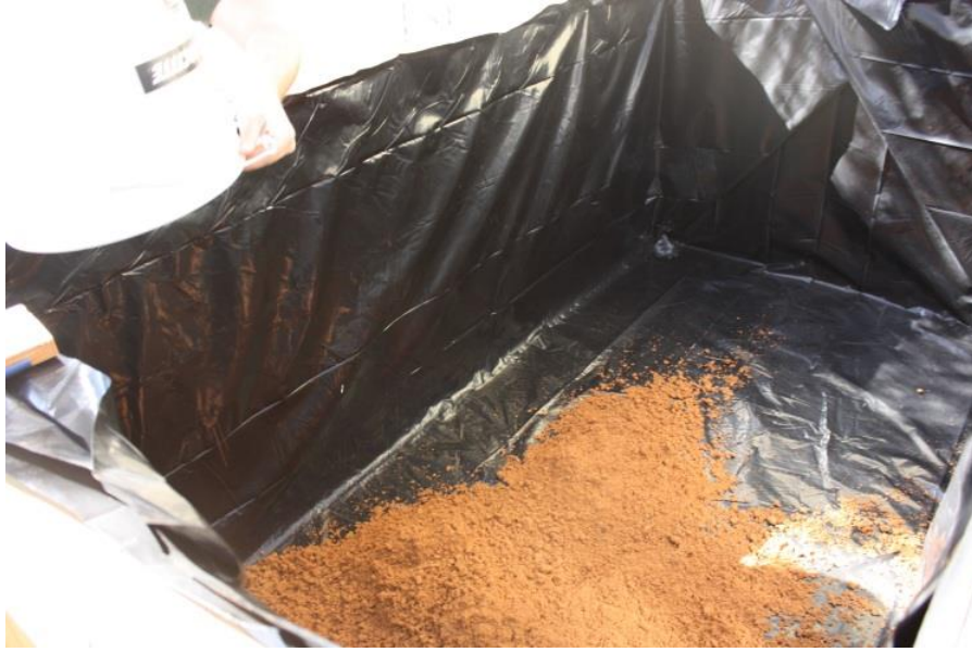
Figure 20. Dumping a batch of backfill in the soil box.
