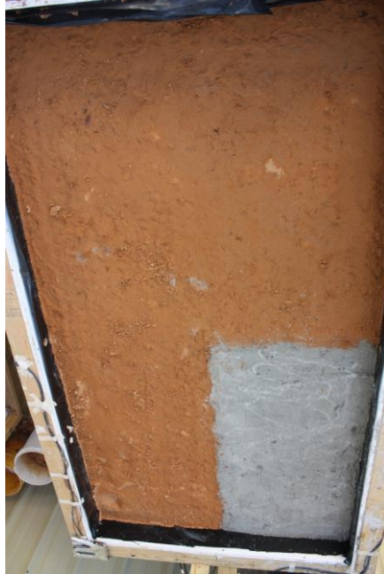
Figure 28. Box completely filled (7/8 of the volume is backfill and 1/8 a simulated void repair with CLSM).
