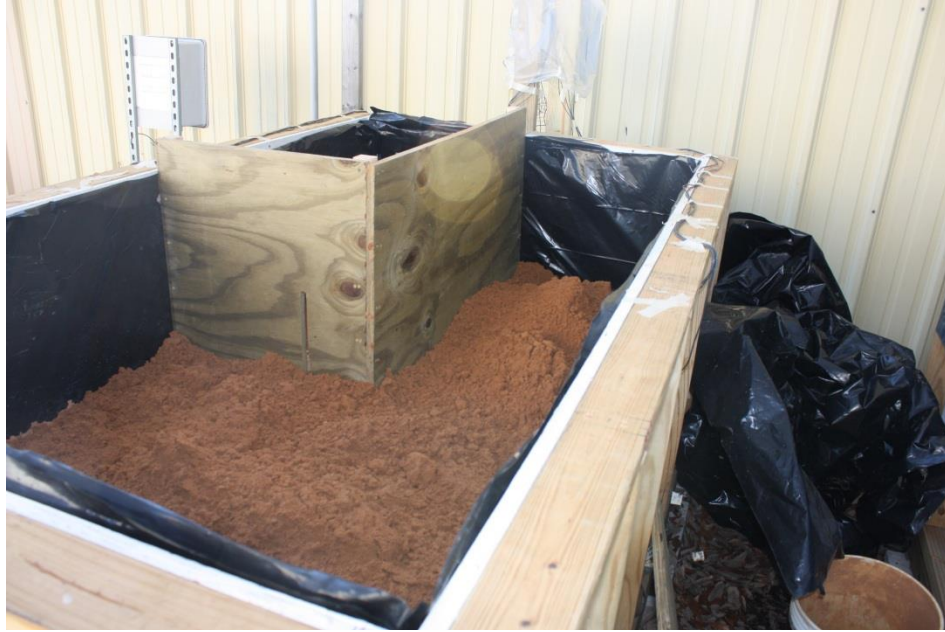
Figure 24. Backfill around the dam.
