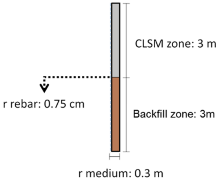
Figure 46. FEM domain geometry for model simulations. Rotational symmetry axis is located at the left.
