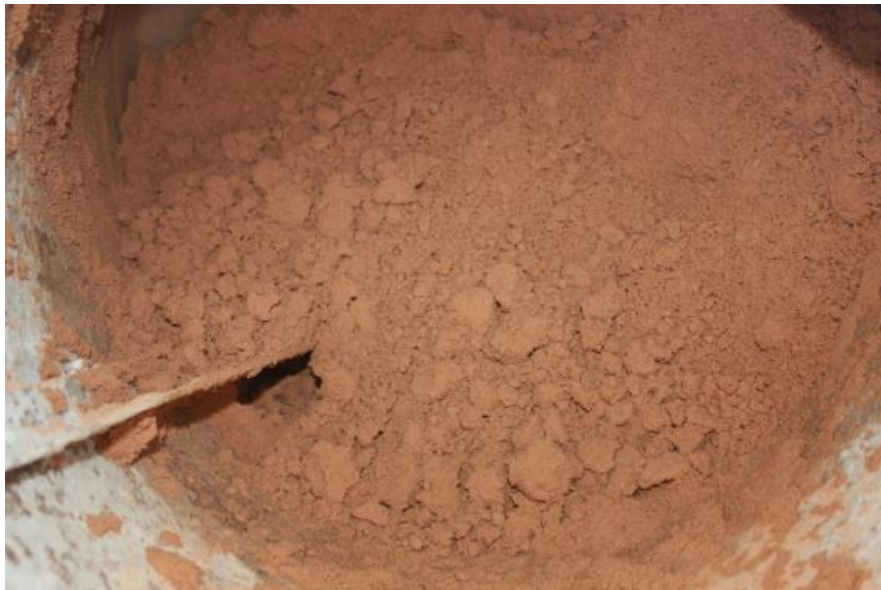
Figure 19. Backfill: mixture of soil with water and sodium chloride.
