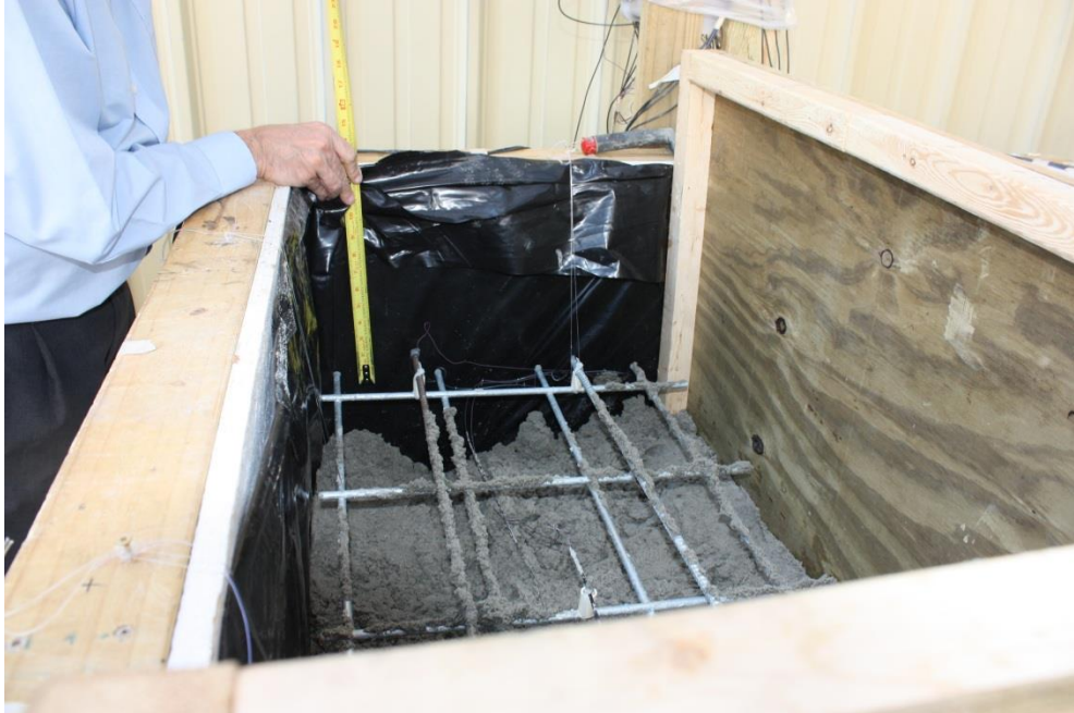
Figure 26. Filling of the simulated void with CLSM.
