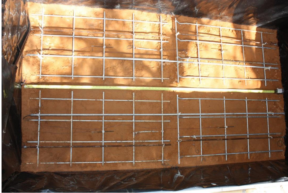
Figure 22. Distribution of specimens in the first layer of the soil box. Front is the right side of the picture.
