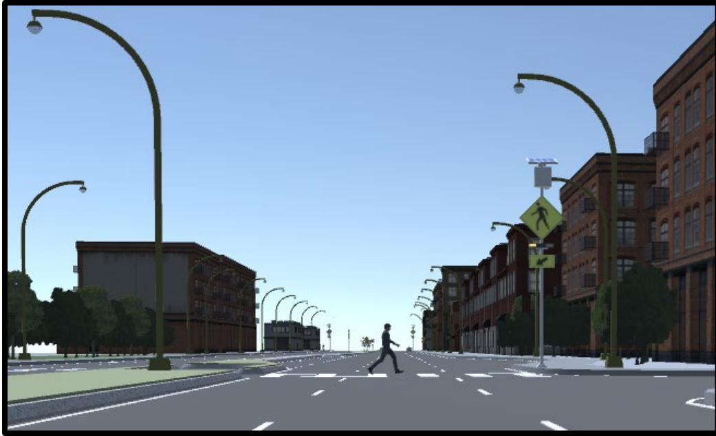
Figure 2 An activated RRFB with a pedestrian crossing
