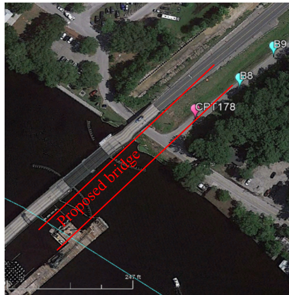
Figure 3-8. Location of soil borings relative to construction Site A3 (Map data © 2021 Google).
