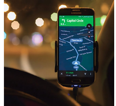
Safely mounted for hands-free operation, a smartphone can emulate an on-board unit to deliver traffic information to a driver.
