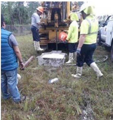
Figure 3-10. Sampling process of the Shelby tubes: (a) drilling, (b) extraction, and (c) wax sealing
