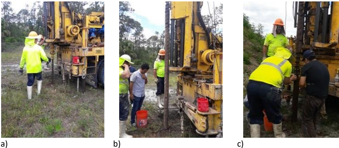
Figure 3-11. Sampling process retrieved from the drill auger. (a) drilling, (b) extraction, and (c) wax sealing. Pictures taken on April 10, 2019
