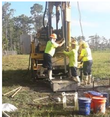
Figure 3-10. Sampling process of the Shelby tubes: (a) drilling, (b) extraction, and (c) wax sealing
