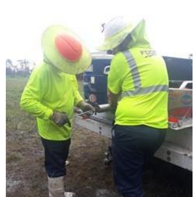
Figure 3-10. Sampling process of the Shelby tubes: (a) drilling, (b) extraction, and (c) wax sealing
