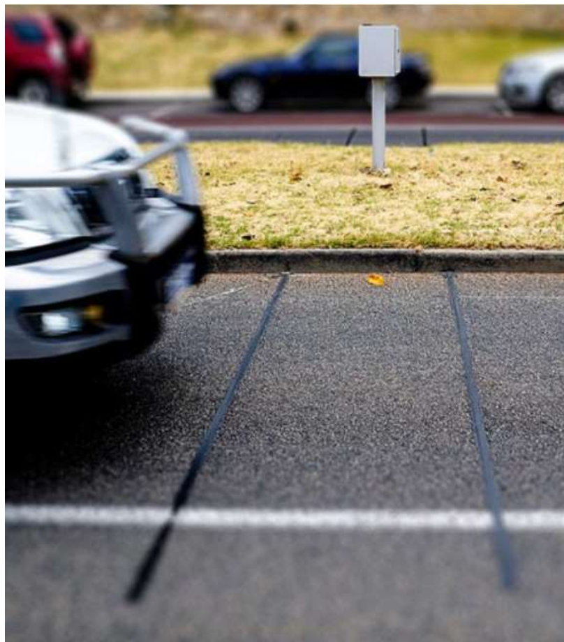
Figure 5: Fixed and Embedded Types of Pneumatic Detectors
