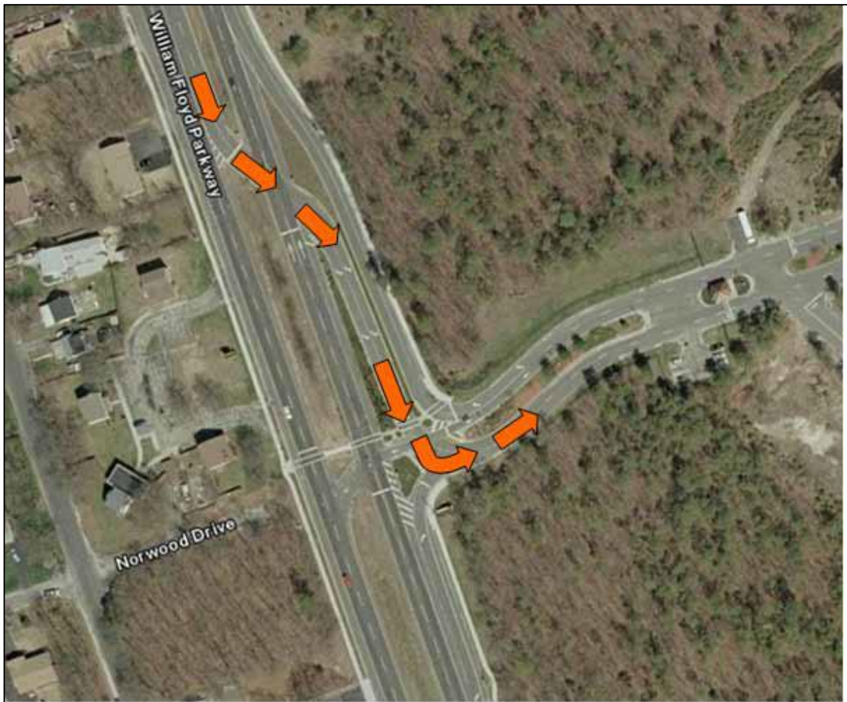
Figure 2-1: Left-turn crossover movement at a three-legged partial CFI in Shirley, New York (Hughes et al., 2010)
