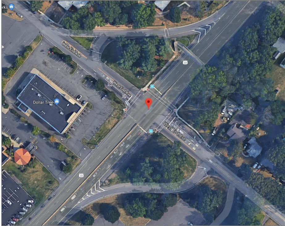
Figure 6-21: Forward/forward jughandle intersection, New Jersey
