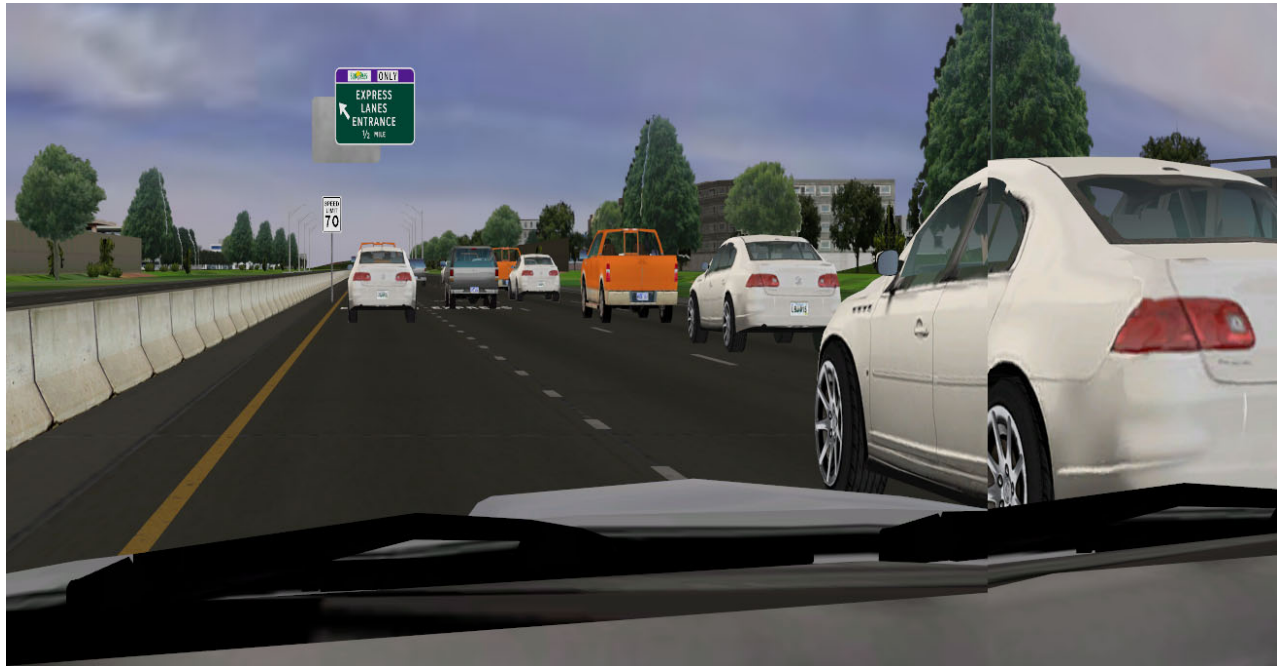
Figure 3-7: Overhead Guide Sign Located at Half Mile from Express Lane Entry
