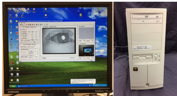
Figure 3-3: Eye-Tracking Computer and Pupil/Corneal Reflection Tracking Software
