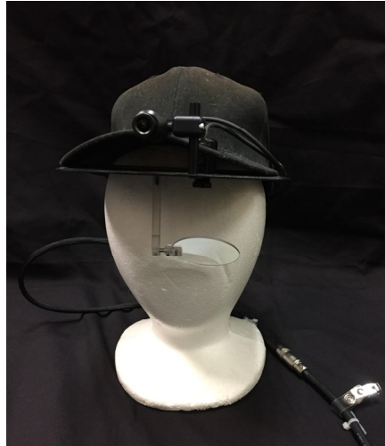
Figure 4-3: ISCAN ETL-500 Eye-Tracker
