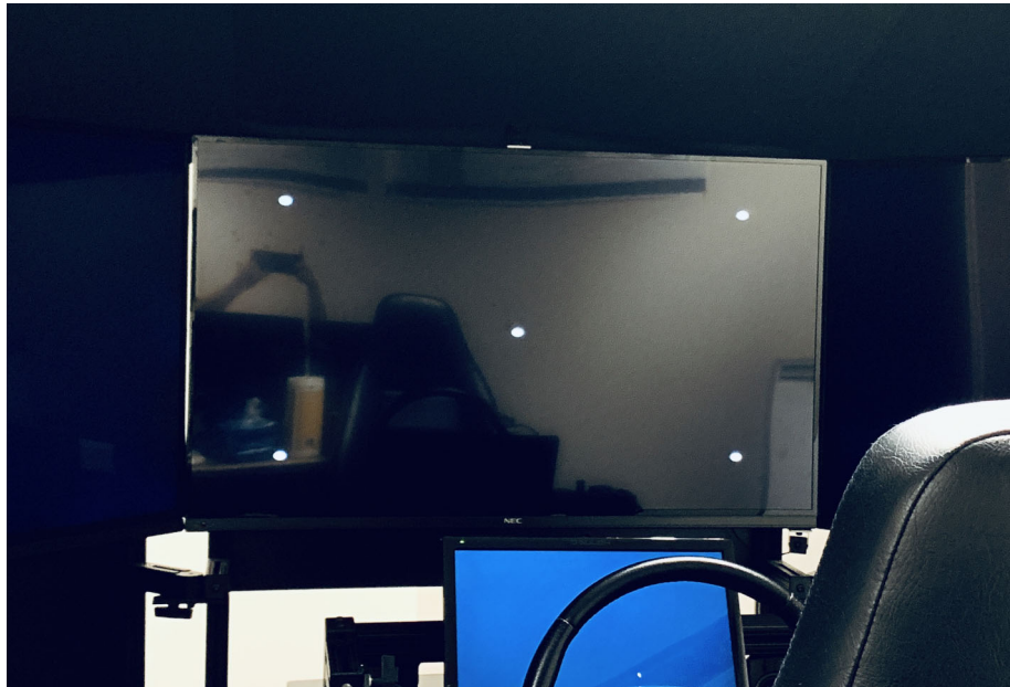
Figure 4-4: Dot Configuration for the Calibration Process
