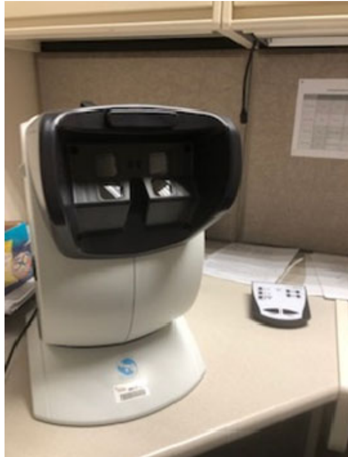
Figure 4-1: Optec Machine Used for Visual Testing and Screening
