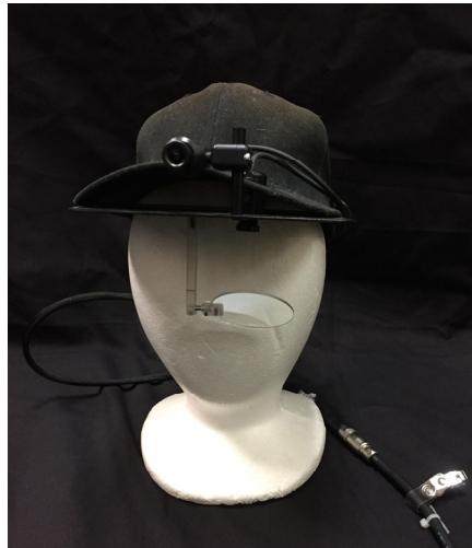
Figure 3-2: ISCAN ETL-500 Eye-Tracker
