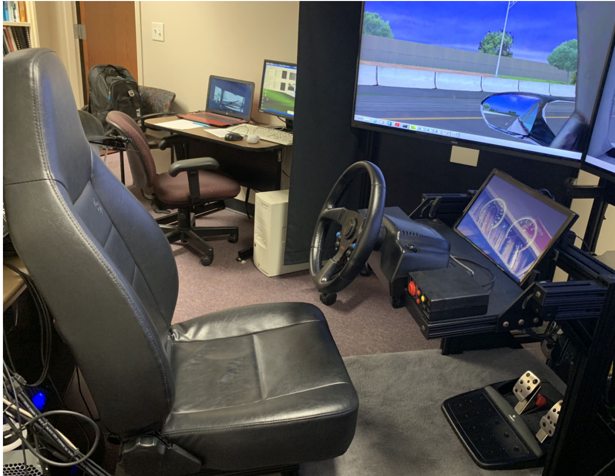
Figure 4-2: UCF NADS Driving Simulator
