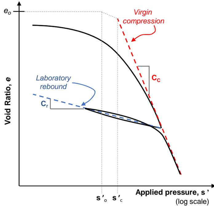
Figure 1-1. Typical consolidation curve of an over-consolidated clay
