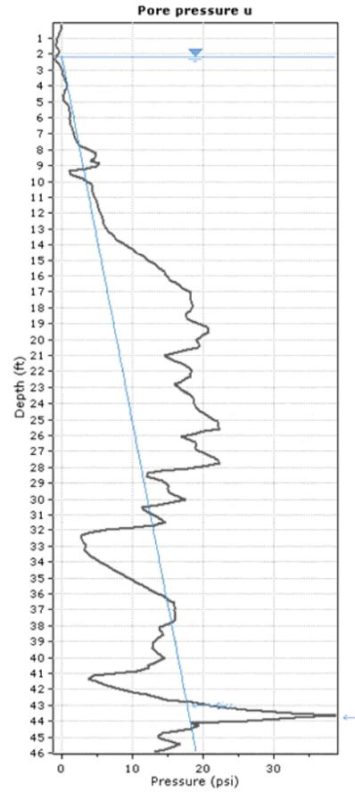
▶ Depth of dissipation test
