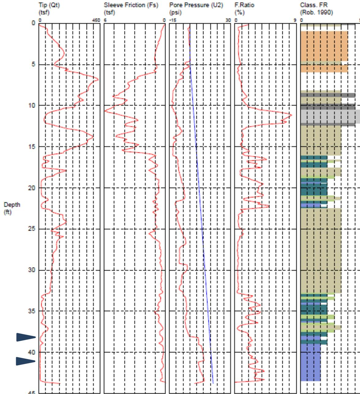
▶ Depth of dissipation test
