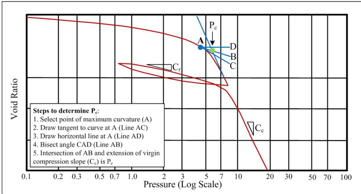
Figure 1-3. Determination of maximum past stress (Source: NAVFAC, 1982)
