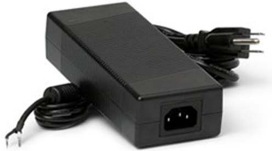
Figure 2-3: 782698-01 NI PS-10 power supply 24 VDC, 5A, 100-120/200-240 VAC
