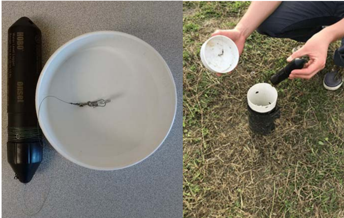
Figure 3.55: Sensor attachment to well cap
