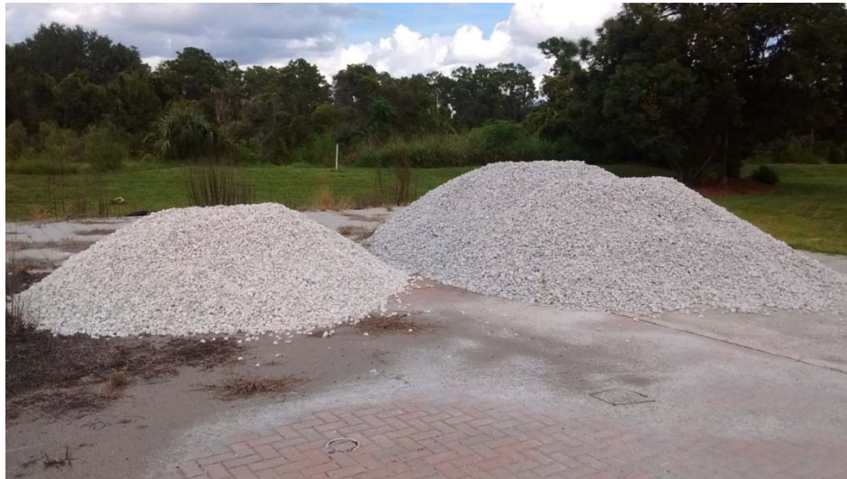
Figure 3.31: No. 4 virgin limestone and No. 4 RCA aggregates
