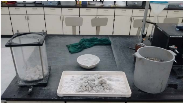
(e) Coating aggregate in fines
