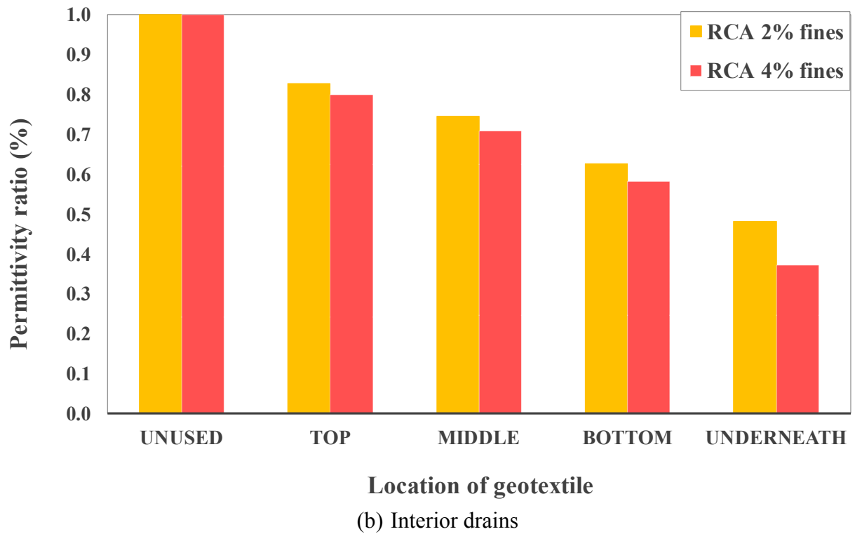
Figure 4.21: Permittivity ratio of in situ geotextiles
