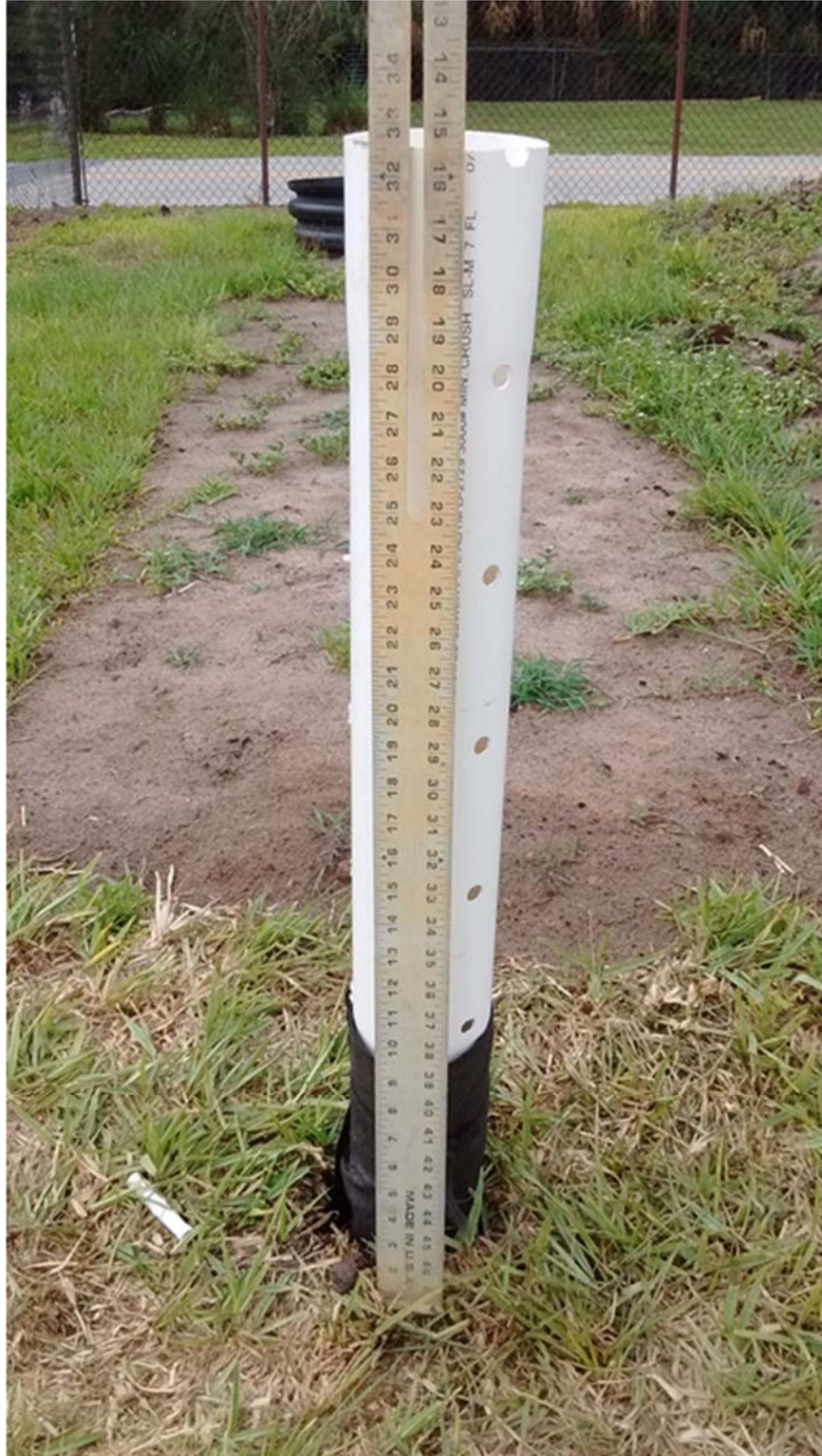
Figure 3.52: Verification of well placement depth
