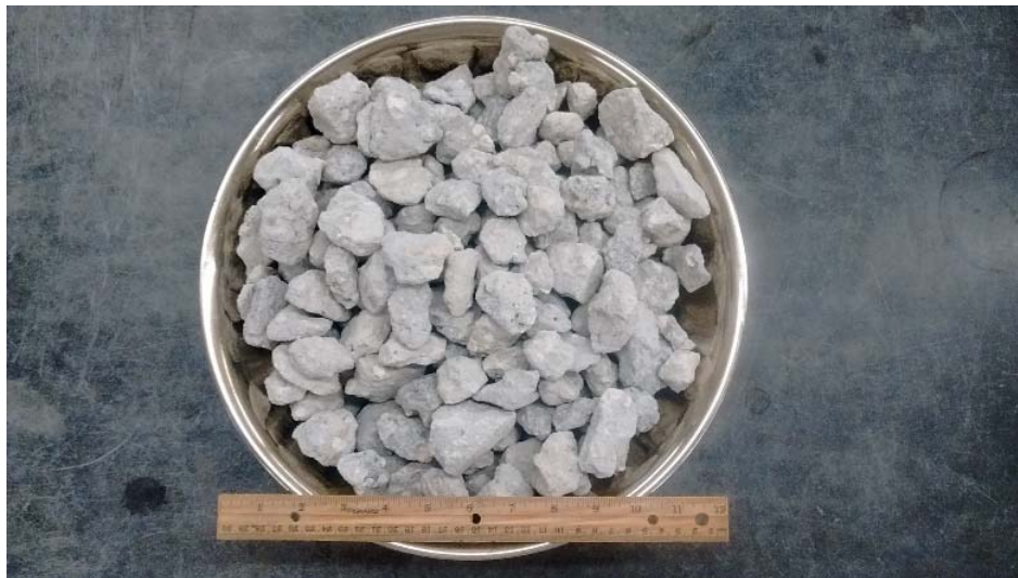
Figure 3.14: RCA aggregate (1-ft ruler used for scale)
