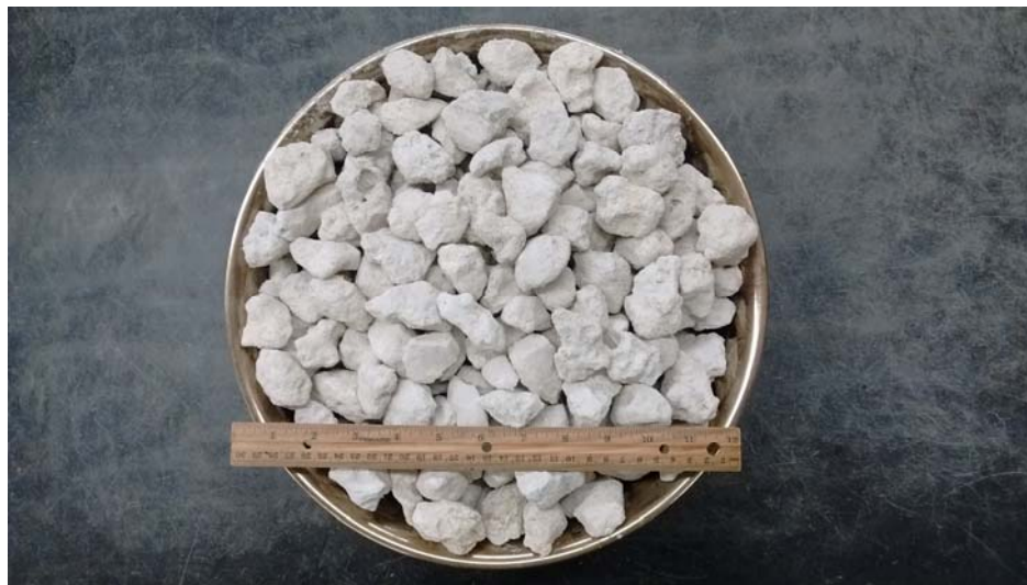
Figure 3.12: Limestone aggregate (1-ft ruler used for scale)
