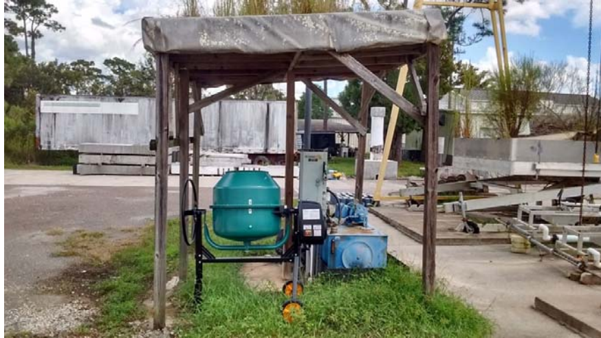
Figure 3.32: Concrete mixer for fines generation prior to the placement of aggregates
