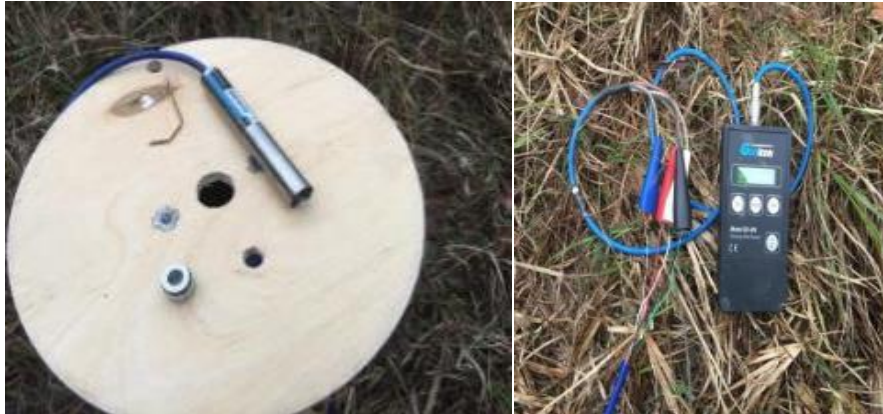
Figure 3-7. (left) Piezometer and rolled cable and (right) Geokon piezo handheld reader
