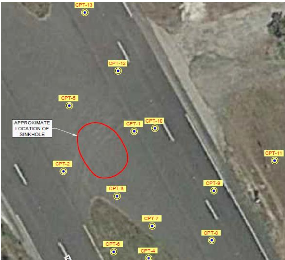
Figure 6-6. CPTs and sinkhole location at US-441 in Marion County (Terracon , 2017)
