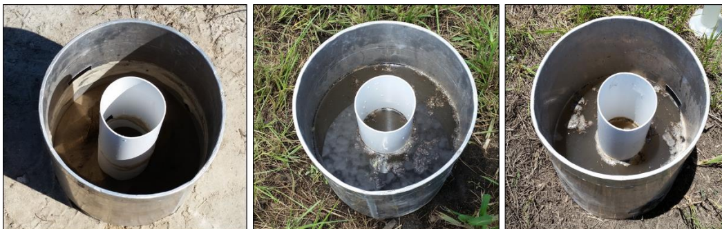
Figure 16: Double ring infiltrometer test at SR 35 Basin 9b (left), SR 35 Basin 2 near inlet (middle), SR 35 Basin 2 center of stormwater basin (right)
