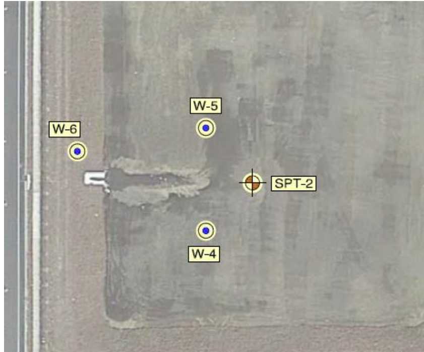
Figure 13: Well locations at SR 35 Basin 2
