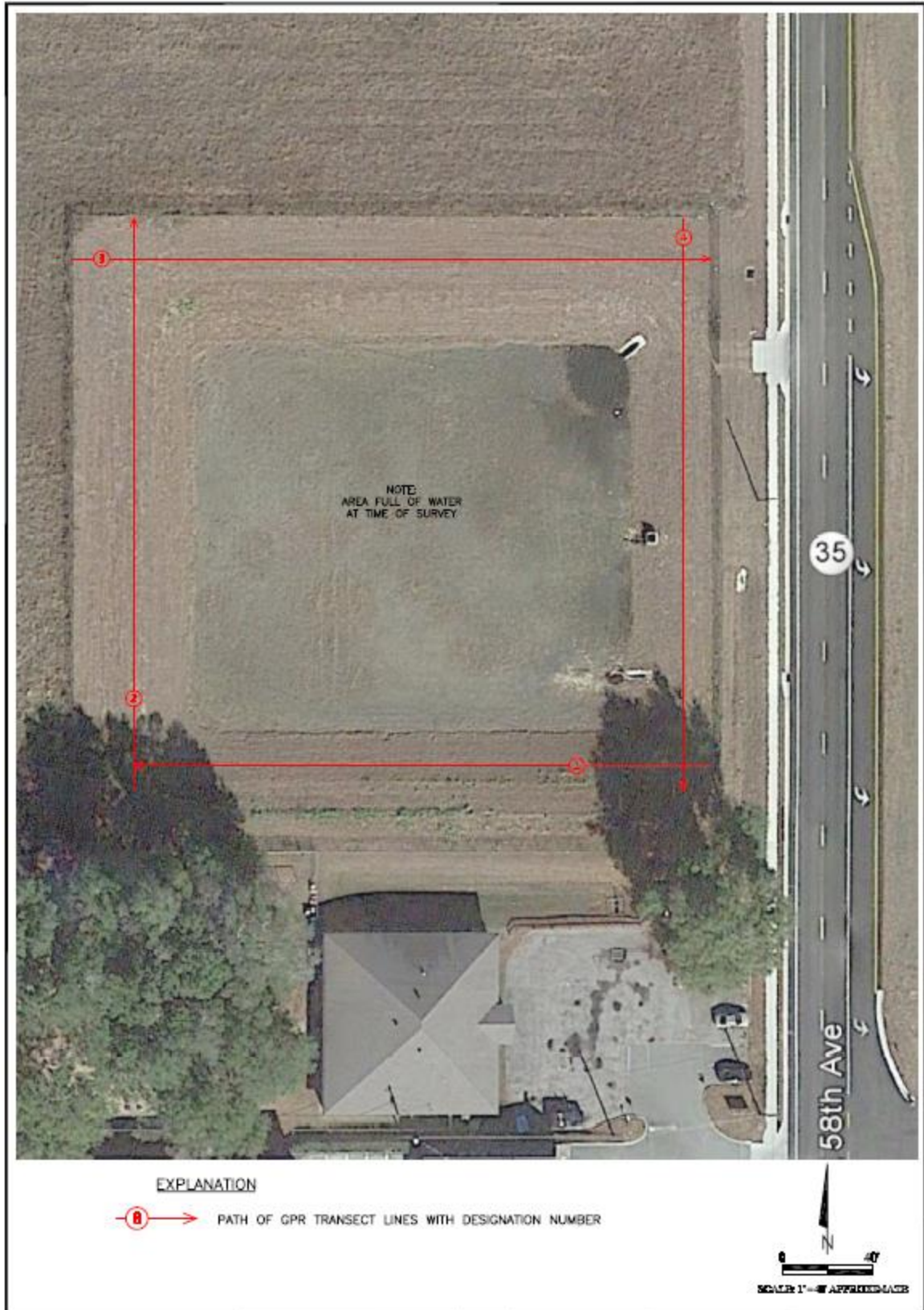
Figure 31: GPR anomalies of SR 35 Basin 3
