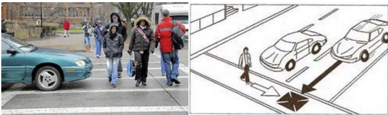
Figure 18: Condition Showing Potential Pedestrian-Vehicle Conflict
