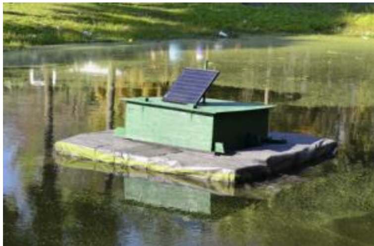
Figure 18: Floating media bed reactor at the East Palatka pond
