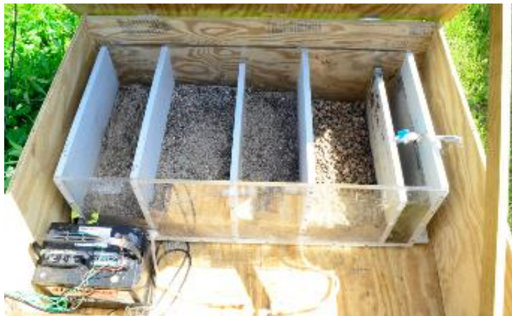
Figure 4: Sloped media bed reactor at Zolfo Springs pond
