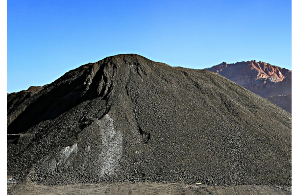
Nationwide, stockpiles of recovered asphalt pavement are available for use in new road surfaces.
