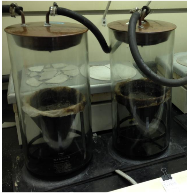
Figure 3-4 Asphalt binder extraction (reflux)
