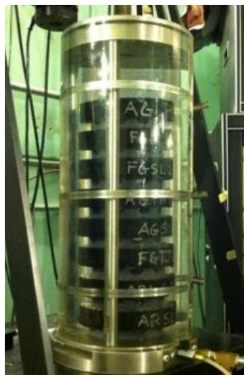
Figure 3-18 Tabletop triaxial chamber (Roque et al, 2013)
