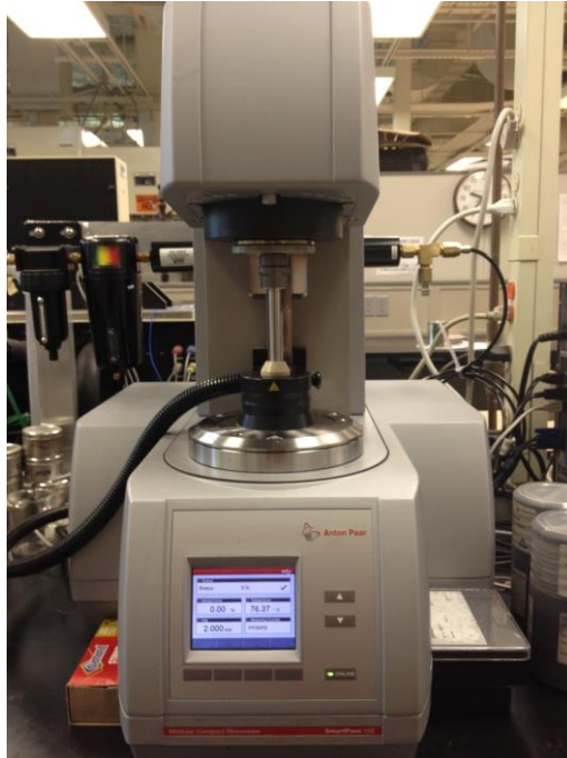
Figure 3-8 MSCR testing device located at FDOT SMO laboratory
