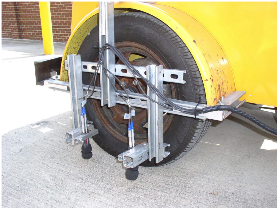
Figure 1. Prototype Test Rig With Intensity Probes, Phase 1
