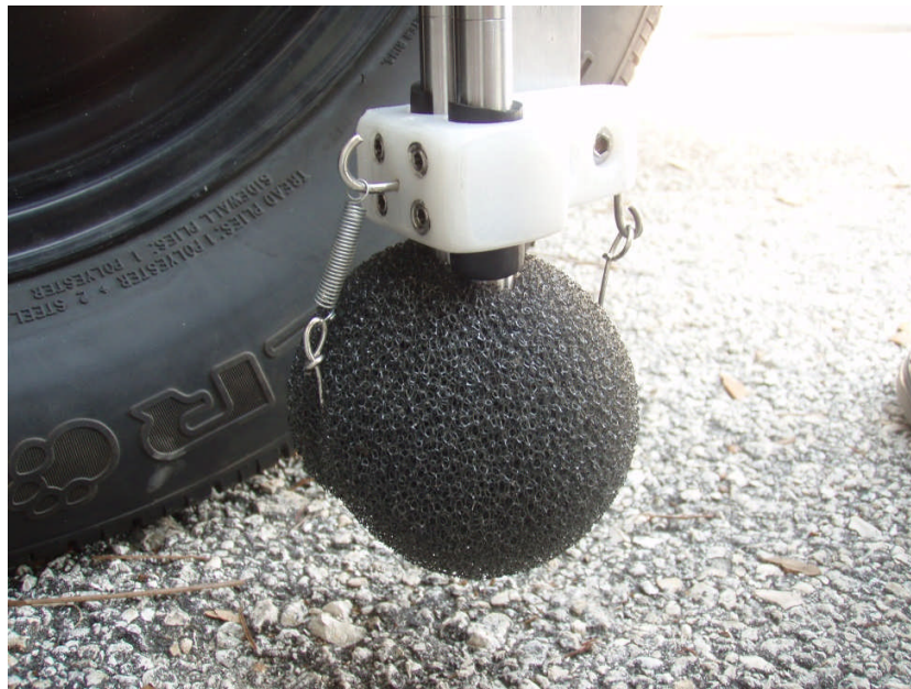
Figure A.1.18. Windscreen placed and secured over two microphones that comprise an intensity probe
