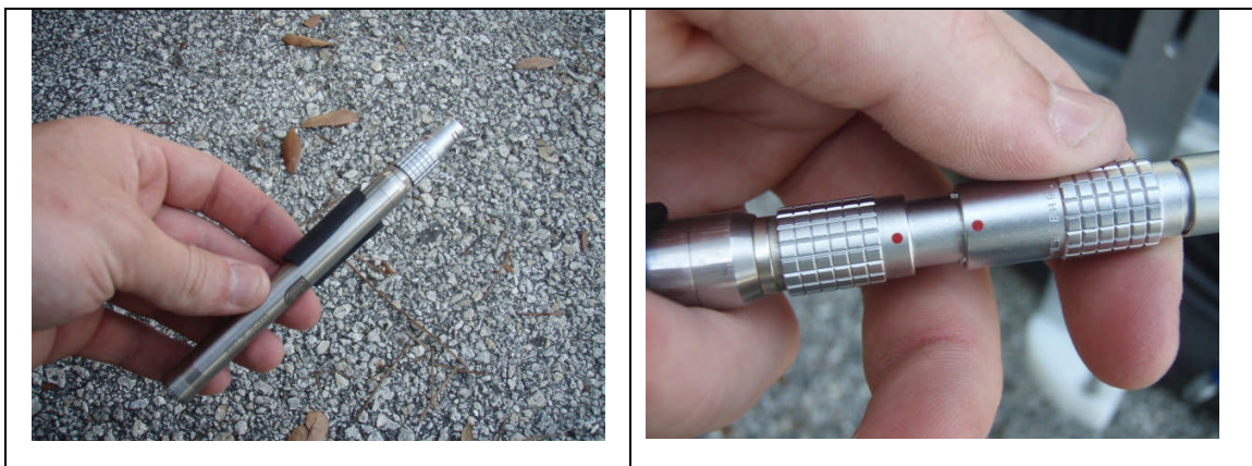
Figure A.1.8. Microphone/preamplifier assembly (left) and proper connection of cable (right)
