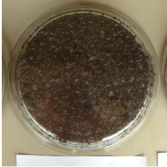
Figure 5.9 - Pie-Plate Test Results for Titan America FC-5 Mix at Optimum Asphalt Content; a) PG 67-22; b) PG 76-22; c) ARB-12
