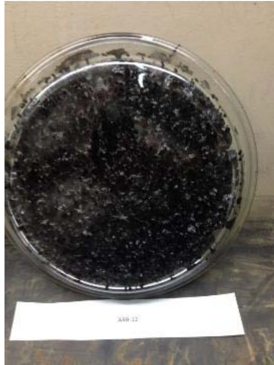
Figure 5.10 - Pie-Plate Test Results for Titan America FC-5 Mix at 0.6% Above Optimum Asphalt Content; a) PG 67-22; b) PG 76-22; c) ARB-12
