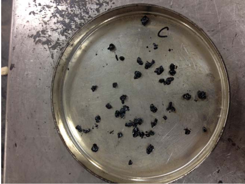
Figure 5.6 – FC-5 Coated Fine Aggregate “Draindown” During from Draindown Testing (AASHTO T 305)
