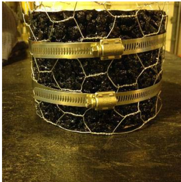
Figure 6.1 – FC-5 Specimen Confined with “Chicken Wire” Prior to Long-Term Aging
