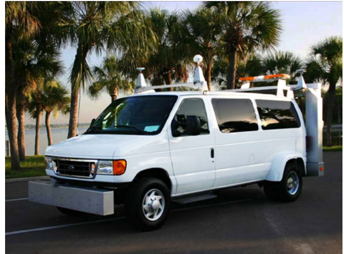
The Pavement Condition Survey is conducted by operators using specially equipped vans.
