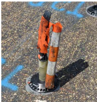
Figure A-5. Sample 3T Failure at 71 Impacts.
