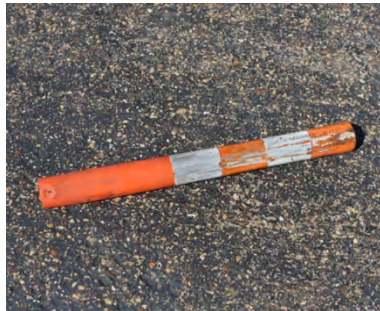
Figure A-2. Sample 1B Failure at 27 Impacts.
