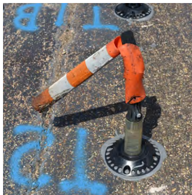
Figure A-3. Sample 2T Failure at 66 Impacts.
