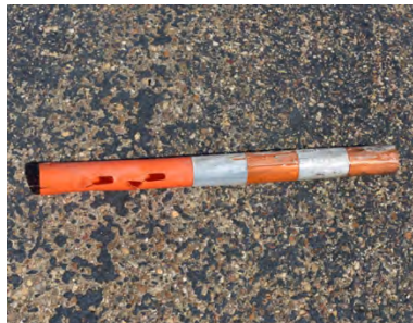
Figure A-6. Sample 3B Failure at 28 Impacts.
