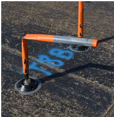
Figure A-15. Sample 8T Failure at 6 Impacts.
