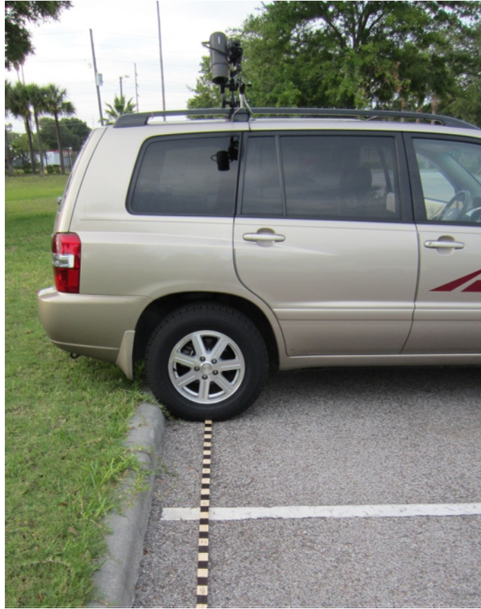
Figure 4-5. Lane-Keeping Video Camera and Calibration Board.
