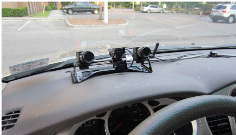
Figure 4-2. Dash-Mounted Eye-Tracking Equipment.
