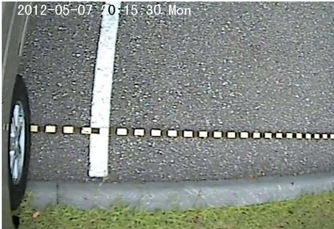
Figure 4-6. Video Image of Calibration Board from Outboard Lane-Keeping Camera.
