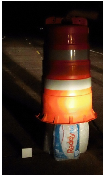
Figure 3-7. Formation of Dew on Surface of Channelizing Drum for Luminance Evaluation.
