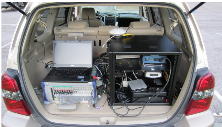
Figure 4-4. Data Collection Equipment in the Instrumented Vehicle.
