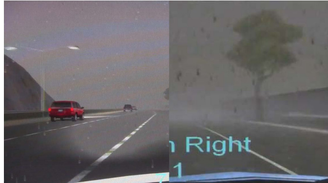
Partial views from the driving simulator show a level 3 (left) and a level 4 (right) rainfall event. The reduced visibility caused drivers to strongly alter their speeds.
