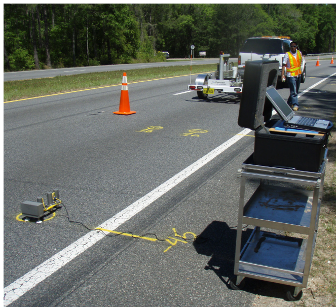
FWD (trailer) and PSPA (bottom left) data were collected both along and between the wheel paths at six positions along this stretch of a North Florida highway.
