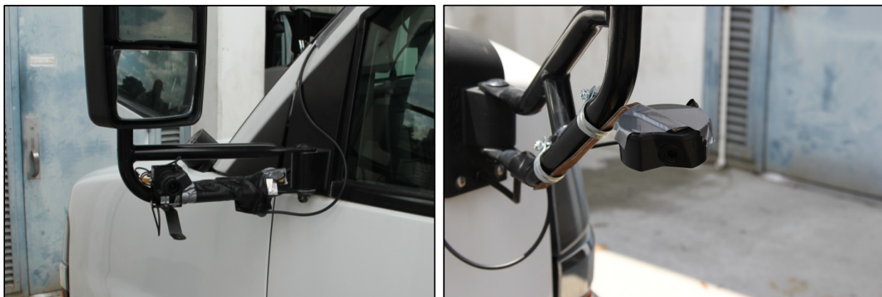
Figure 3-7. Left and right cameras used on the cutaway bus.
