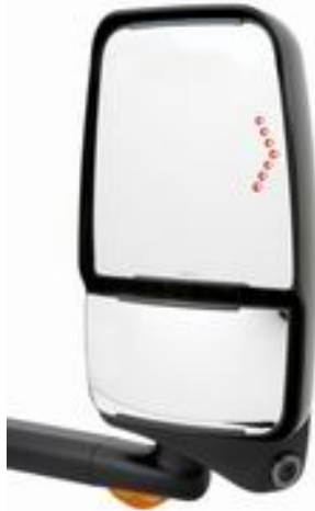
Figure 2-7. Mirror-camera system used for cutaway bus.
