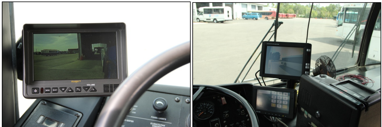
Figure 3-5. Left and right side monitors on type A bus.
