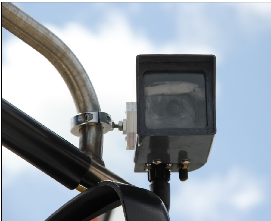
Figure 4-3. Right side camera installed on type A bus.
