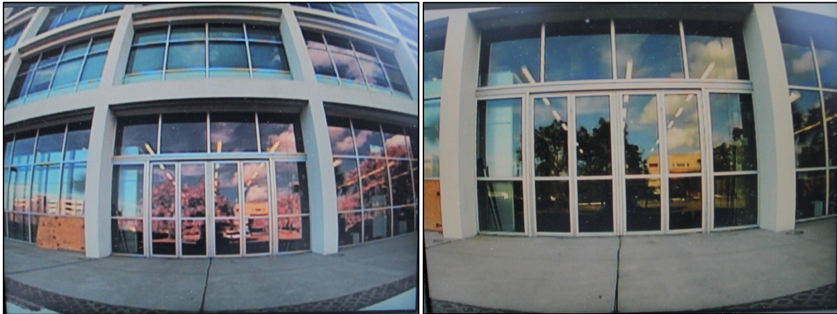
Figure 2-1. View from 100° angle lens (left) and 65° angle lens (right).
