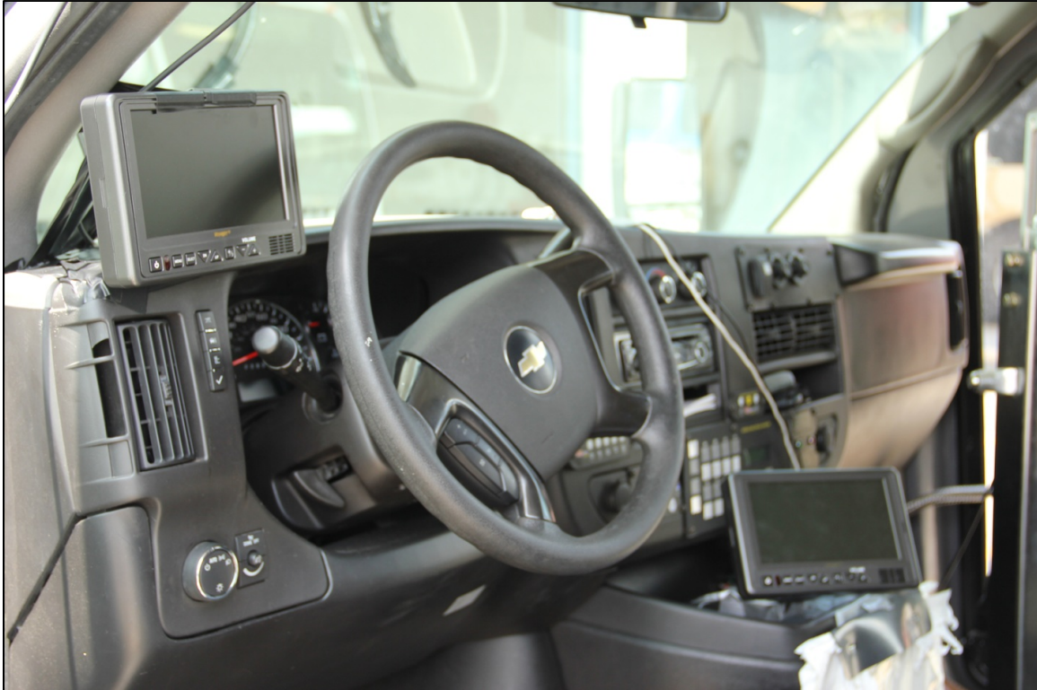
Figure 3-8. Left and right side monitors mounted on the cutaway bus.
