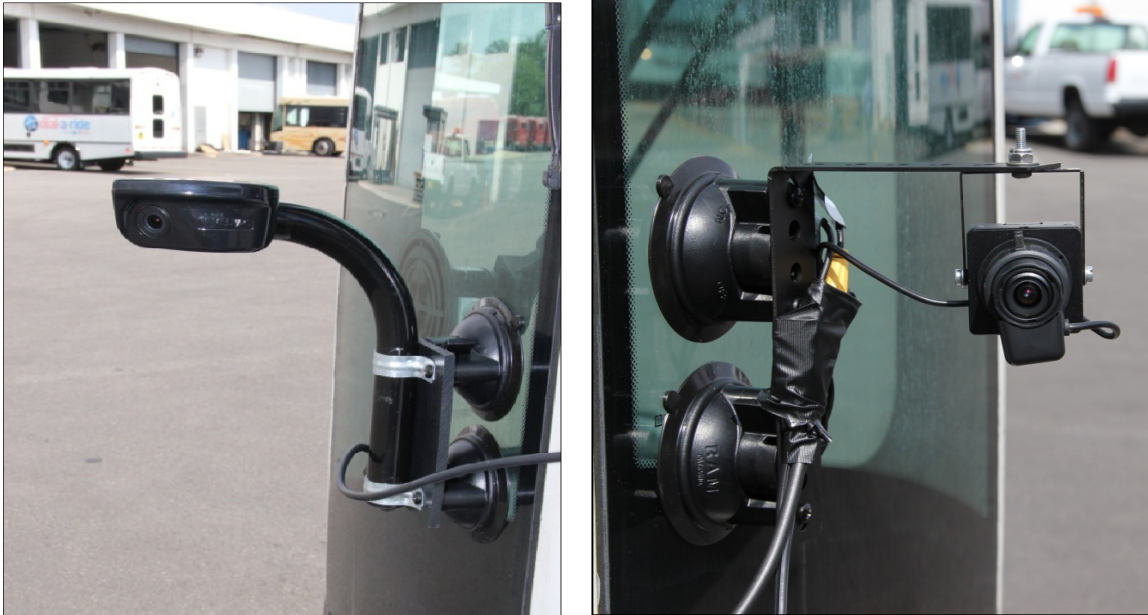
Figure 3-4. Left and right side cameras on type A bus.
