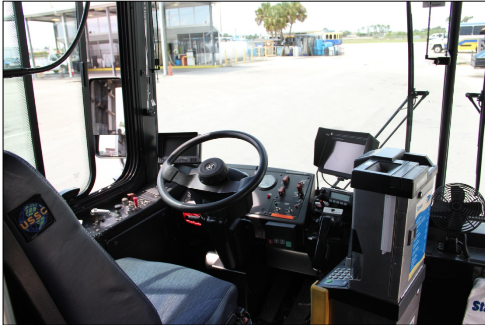
Figure 4-4. Monitors installed in the type A bus.
