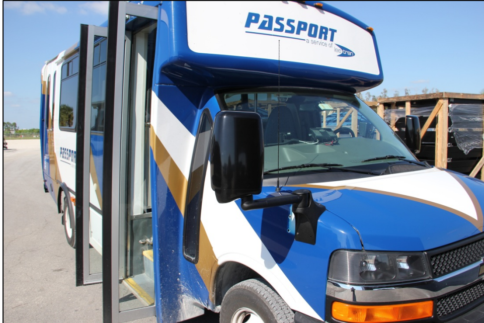
Figure 4-6. Right side mirror-camera system.
