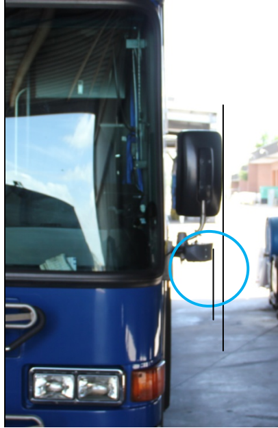
Figure 4-2. Clearance between camera and mirror outline.
