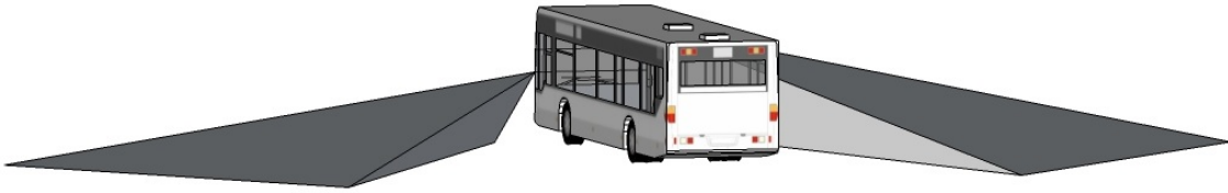
Figure 1-2. Three-dimensional area blind to the driver (blind zone).
