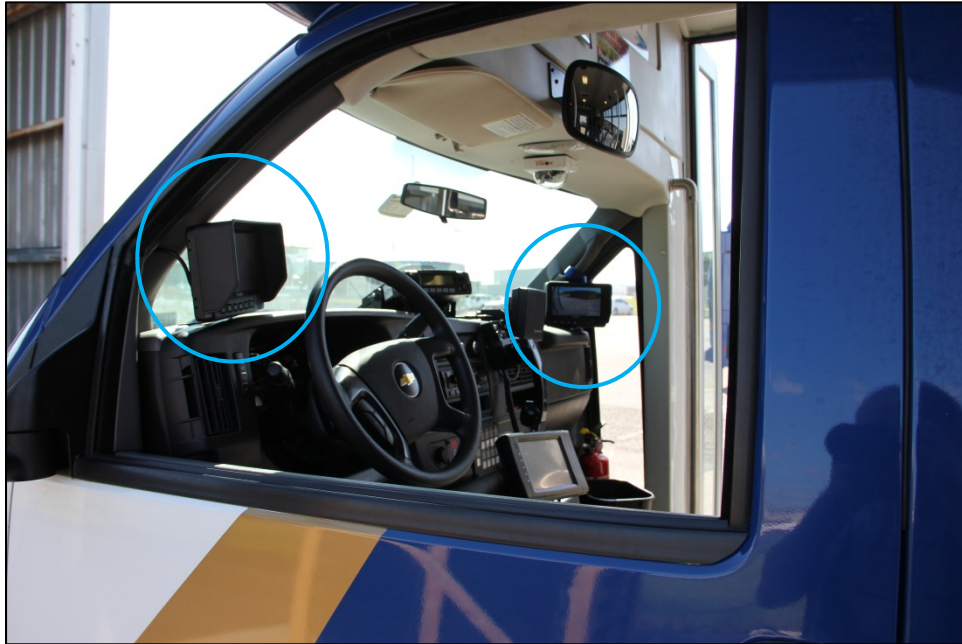
Figure 4-8. Monitors installed on dashboard of cutaway bus.
